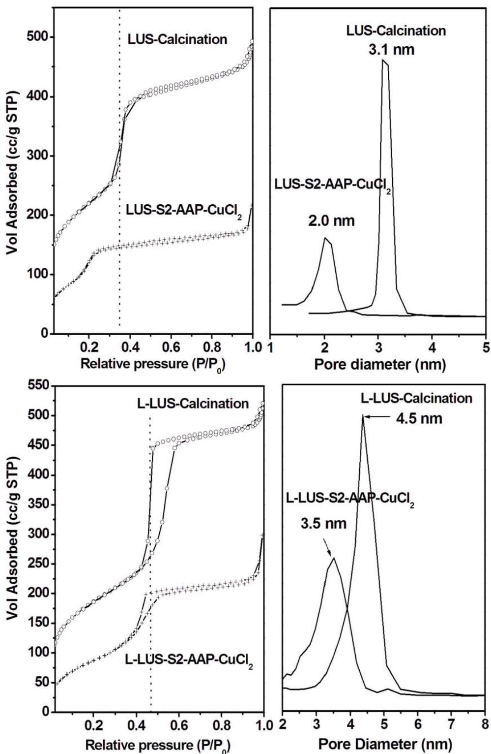
Figure 5.12 N<sub>2</sub> adsorption-desorption isotherms (left) and pore size distribution from BJH method (right) of the final samples.
