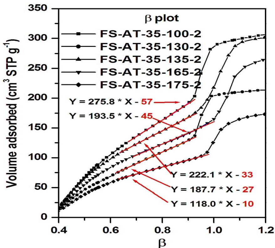
Figure 3.22  $\beta$ -plots of FS-AT-35-X-2 silicas
