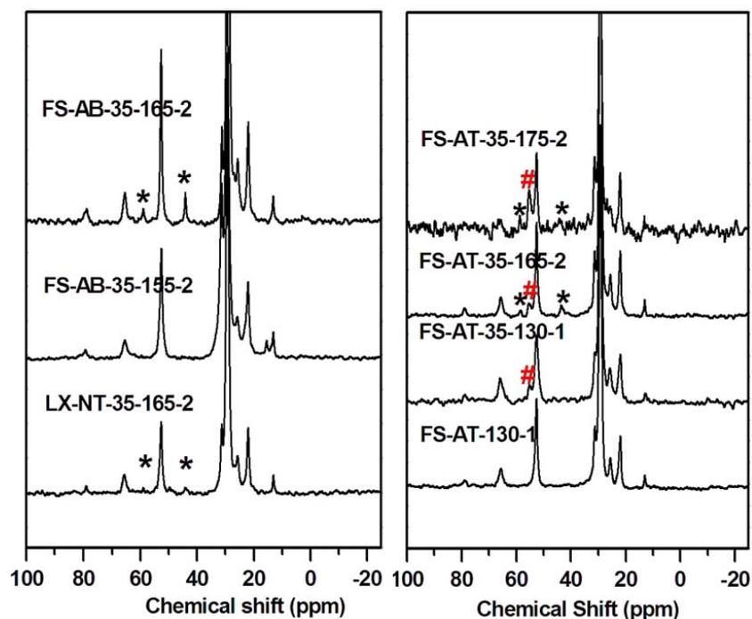
Figure 3.27  $^{13}\text{C}$  CP MAS NMR spectra of FS-AB-35-X-2 and LX-NT-35-165-2 (left), FS-AT-X (right); (\*) Chemical shift of species generated by decomposition of surfactants, (#) chemical shift of TMA.
