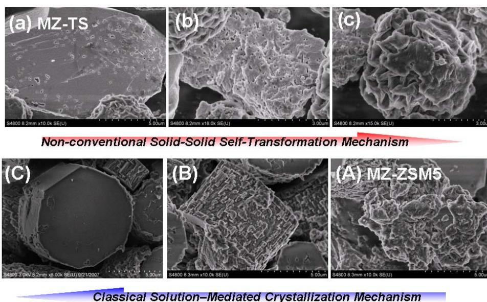
Scheme 4.1 Formation mechanism of crystalline hybrid materials using  $\text{CTA}^+$  using  $\text{TPA}^+$  as co-temple in the present work.
