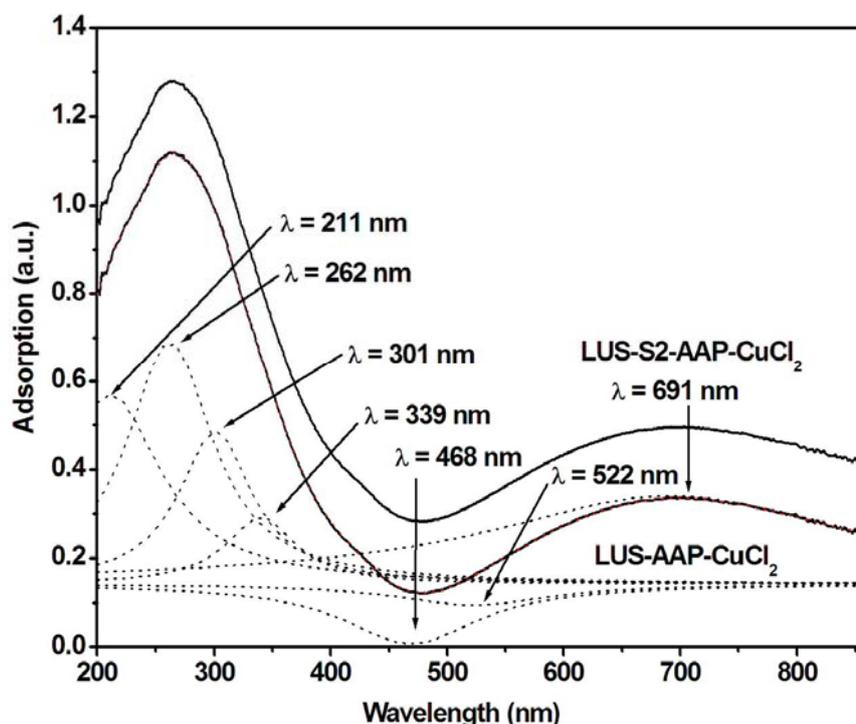
Figure 5.7 UV-vis spectra of LUS-Sn-AAP-CuCl<sub>2</sub> series, dot lines are obtained by Lorentzian multipeak fitting.
