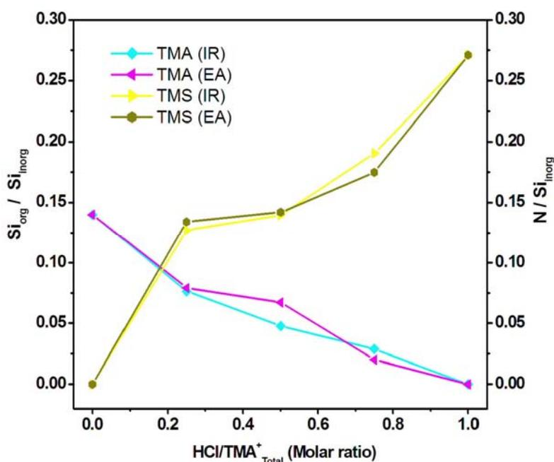
Figure 5.5 Variarion of TMS and TMA concentrations versus the HCl/TMA molar ratio, IR and EA indicate that data were derived from IR spectroscopy and elemental analysis, respectively.
