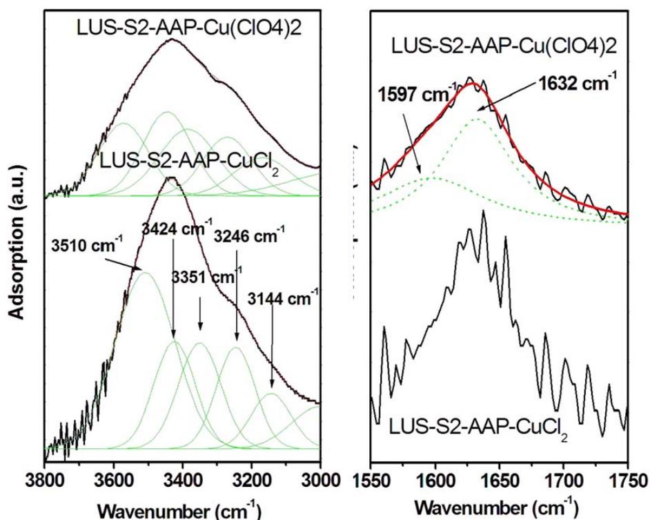
Figure 5.17 FT IR spectra of samples LUS-S2-AAP-CuCl<sub>2</sub> and LUS-S2-AAP-Cu(ClO<sub>4</sub>)<sub>2</sub>: O-H and N-H stretching frequency range (left) and deformation range (right).
