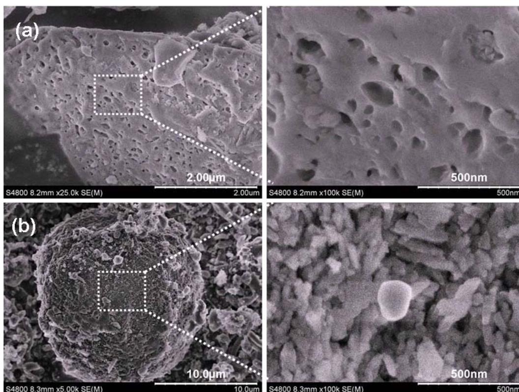
Figure 4.14 SEM images of calcined hybrid materials containing Ti atom synthesized using CTATos and TPA as co-template (Si/Ti=30): a) well facteded particle (rare phase), on the left, zoom of the region indicated by the dot lines, and b) particles of typically 15 μm, on the right, zoom of the region indicated by the dot lines.
