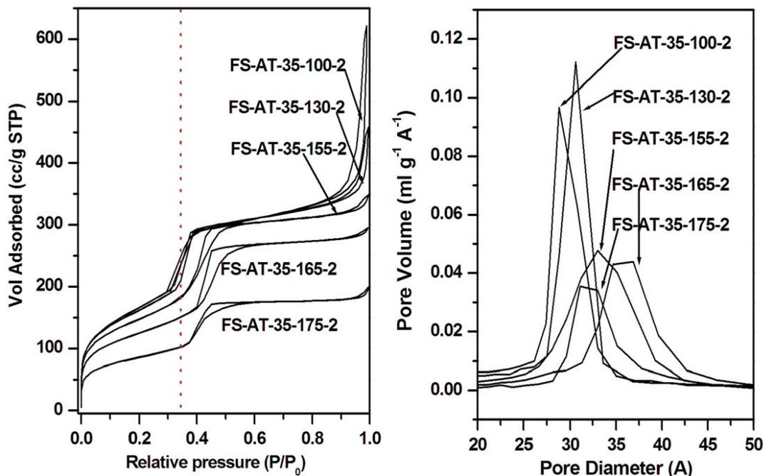
Figure 3.18 N<sub>2</sub> adsorption isotherm (left) and BJH mesopore size distribution (right) from adsorption branch of FS-AT-35-X-2 silicas (see figure 3.17).
