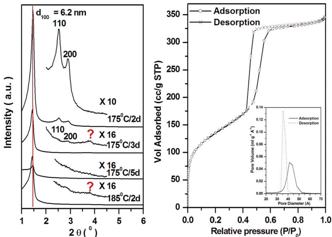
Figure 4.1 XRD patterns of sample FS-TMA-X-2 series synthesized at high temperature (left) and N<sub>2</sub> adsorption-desorption isotherm of FS-TMA-175-2 synthesized at 175°C for 2d (right).
