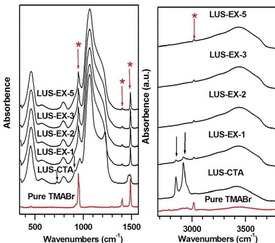
Figure 5.1 FT IR spectra of LUS-1 sample exchanged by  $\text{TMA}^+$  cations, EX stands for abbreviation of 'exchange and the last number for the number of exchange operations.
