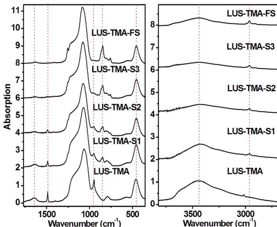
Figure 5.4 FT IR spectra of LUS-1 samples using  $\text{TMA}^+$  (cetyltrimethylammonium) as a patterning molecule via the controlled silylation (in  $\text{Sn}$ ,  $n$  stands for the percentage of total  $\text{TMA}^+$  molecules removal by 1.0 M HCl in ethanol)
