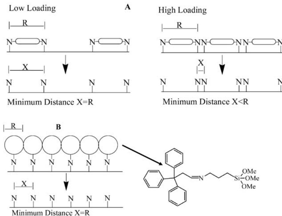
Scheme 2.4 “molecular imprinting” strategy used to synthesize heterogeneous catalyst with isolated active site: A, according to Wulf et al.<sup>78, 79</sup> and B, according to Jones et al.,<sup>84 85</sup>
