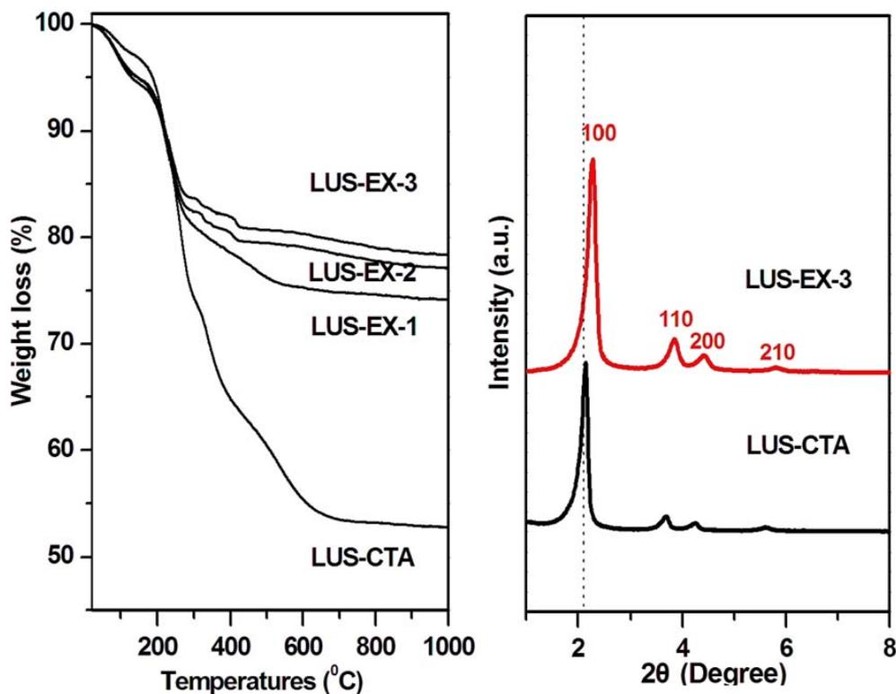
Figure 5.3 TG analysis (left) and XRD patterns (right) of LUS-1 sample exchanged by  $\text{TMA}^+$  cations, EX stands for abbreviation of 'exchange and the last number for the number of exchange operations.
