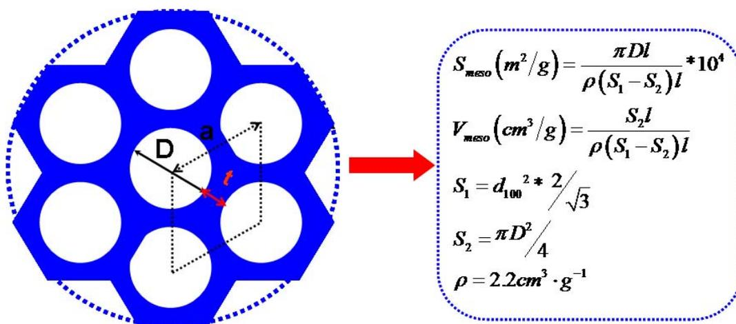
Figure 3.10 Cylindrical geometrical model and related calculation formulas
