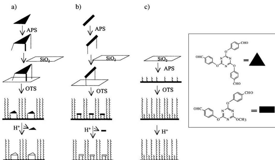
Scheme 2.5 Developed "molecular imprinting" process,<sup>60, 82-83</sup>
