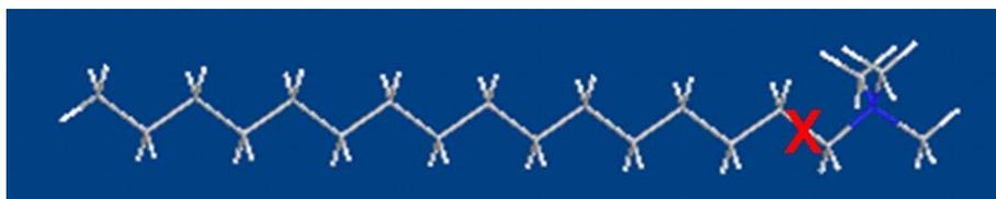
Scheme 5.3 Cetyltrimethylammonium ion (CTA<sup>+</sup>) with a longer tail used as template reagent in [S<sup>+</sup>I] type synthetic pathway of MCM-41 silica.
