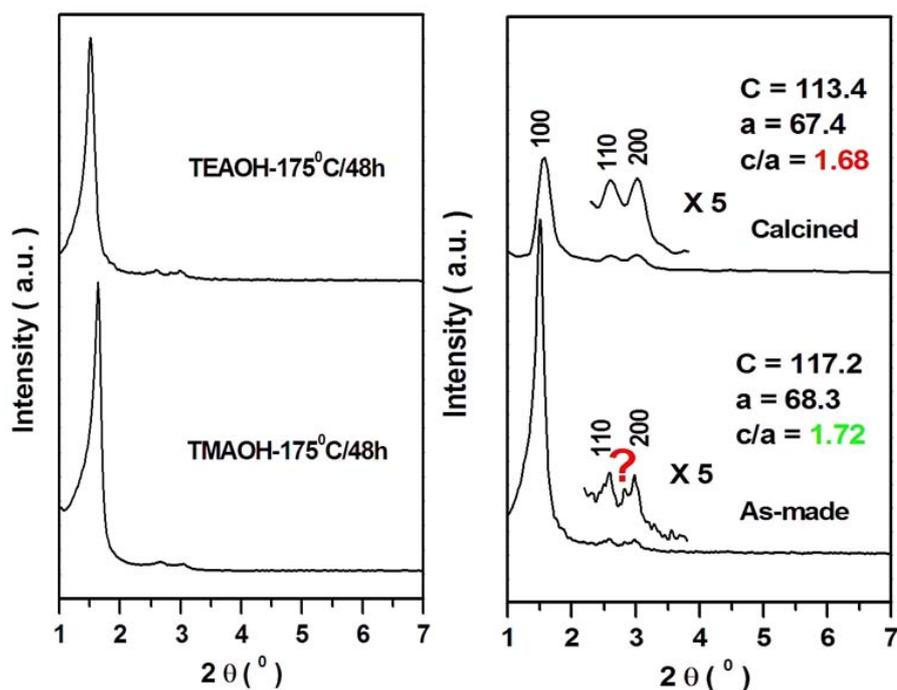
Figure 4.4 XRD patterns of mesophase silicas synthesized using different base sources (left) and XRD patterns of hypothetical SBA-2 mesophase ( $p6_3/cmm$  symmetry) before and after calcination (right)
