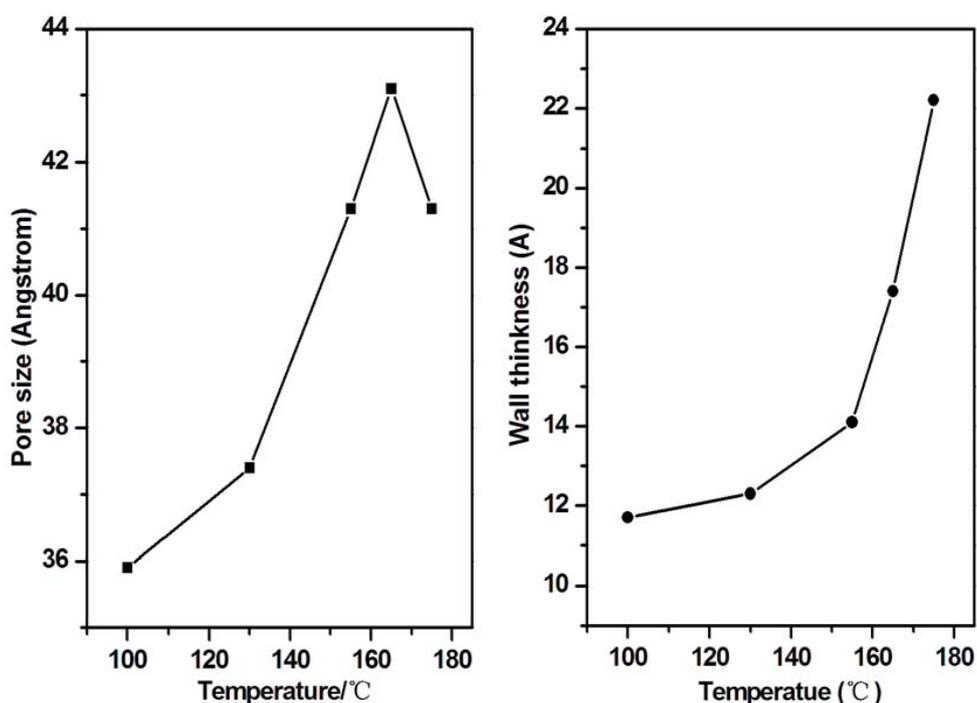
Figure 3.20 Evolutions of pore size (left) and pore wall thickness calculated using BDB method from desorption branch (right) of FS-AT-35-X-2 silicas.
