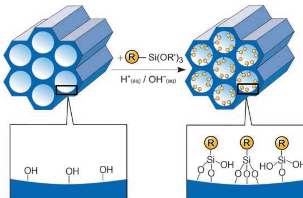
Figure 2.10 Grafting (postsynthetic functionalization) for organic modification of mesoporous pure silica phases with terminal organosilanes of type  $(\text{R}'\text{O})_3\text{SiR}$ . R'=organic functional group
