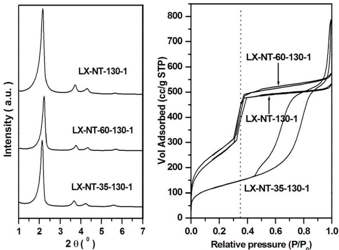
Figure 3.15 XRD patterns (left) and N<sub>2</sub> adsorption-desorption isotherms of samples LX-NT-130-1, LX-NT-60-130-1, and LX-NT-35-130-1 (right).
