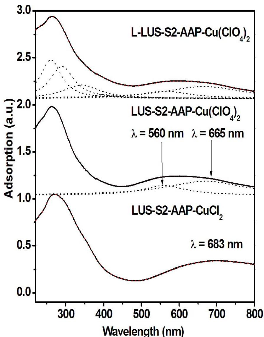
Figure 5.14 UV-vis characterization of LUS-Sn-AAP-CuCl<sub>2</sub>/Cu(ClO<sub>4</sub>)<sub>2</sub> series, dot lines are obtained by Lorentzian multipeak fitting.
