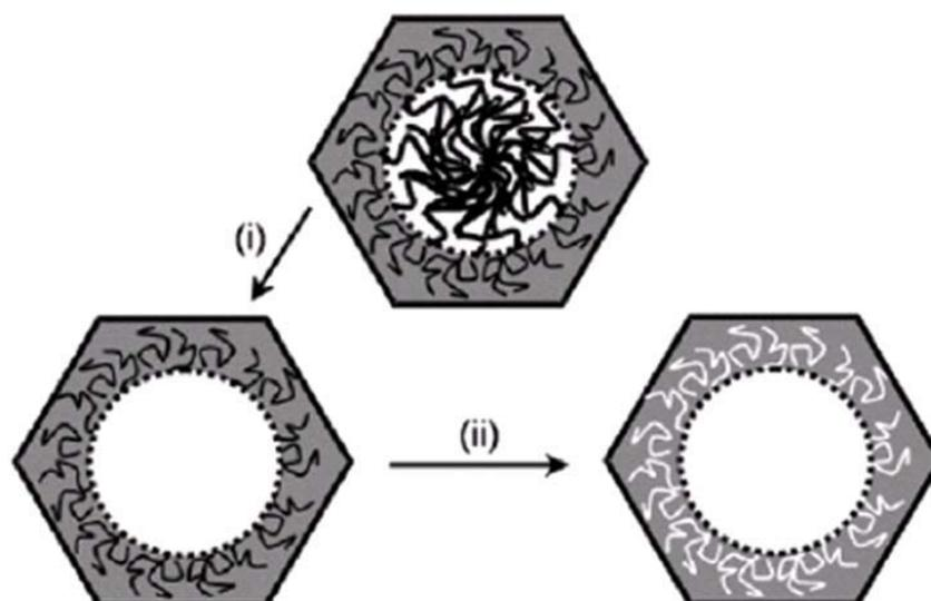
Figure 2.6 Scheme of different states of SBA-15 with PEO surfactant (top), after extraction of surfactants (left) and after calcination (right)<sup>34</sup>
