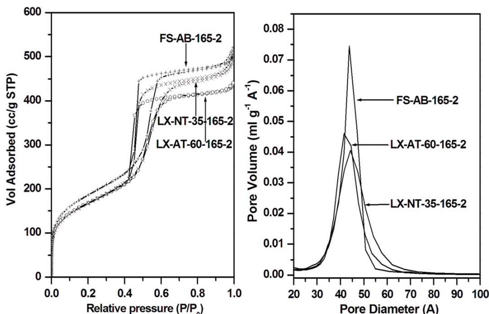
Figure 3.30 N<sub>2</sub> adsorption isotherms of as-made MCM-41 silicas synthesized using different gel composition and aging temperature; (\*) lamellar phase.
