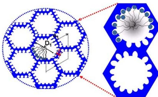
Figure 3.1 Scheme of proposed wall structure for MCM-41 type of silica with open micropores around the hexagonally packed channel (on the right, zoom of two channels).
