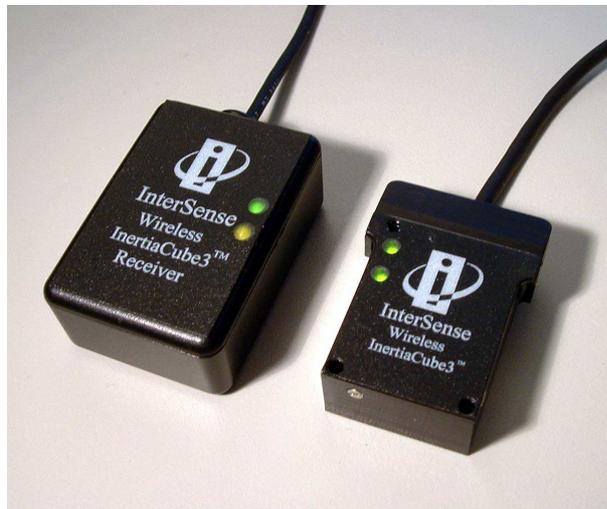
Figure 2.2: Wireless inertiaCube 3: the receiver and the marker [Intersense, 2006].
