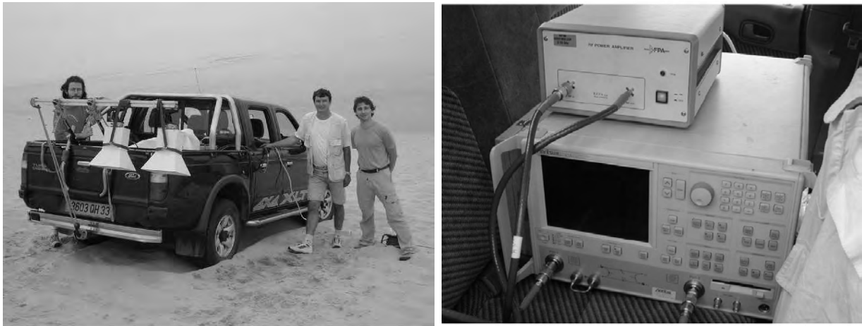
FIG. 4.26 – Bistatic system equipped with two horn antennas during field experiment (left) and connected to a network analyzer ANRITSU 37325A (right) equipped with a time domain function.
