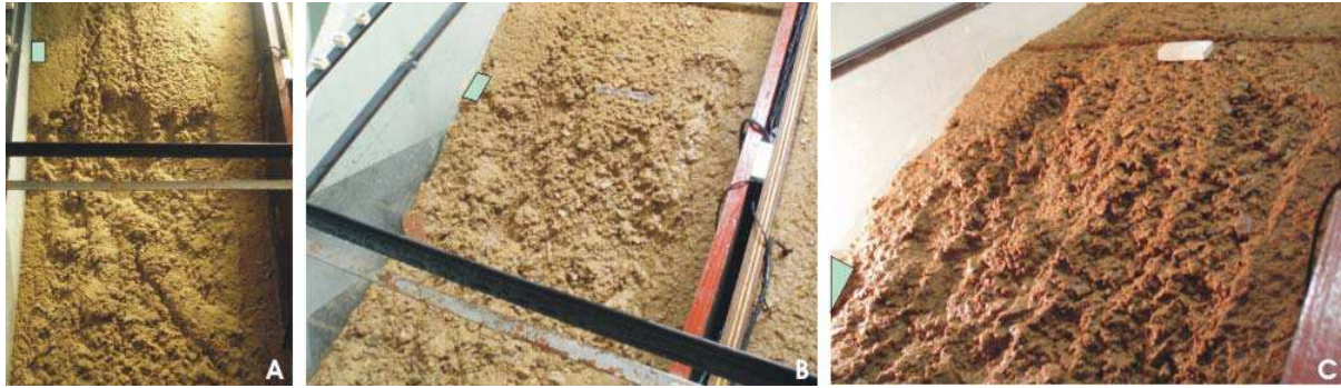
Headward erosion process illustrated from pictures of cycles 3 (A), 5 (B) and 6 (C).
