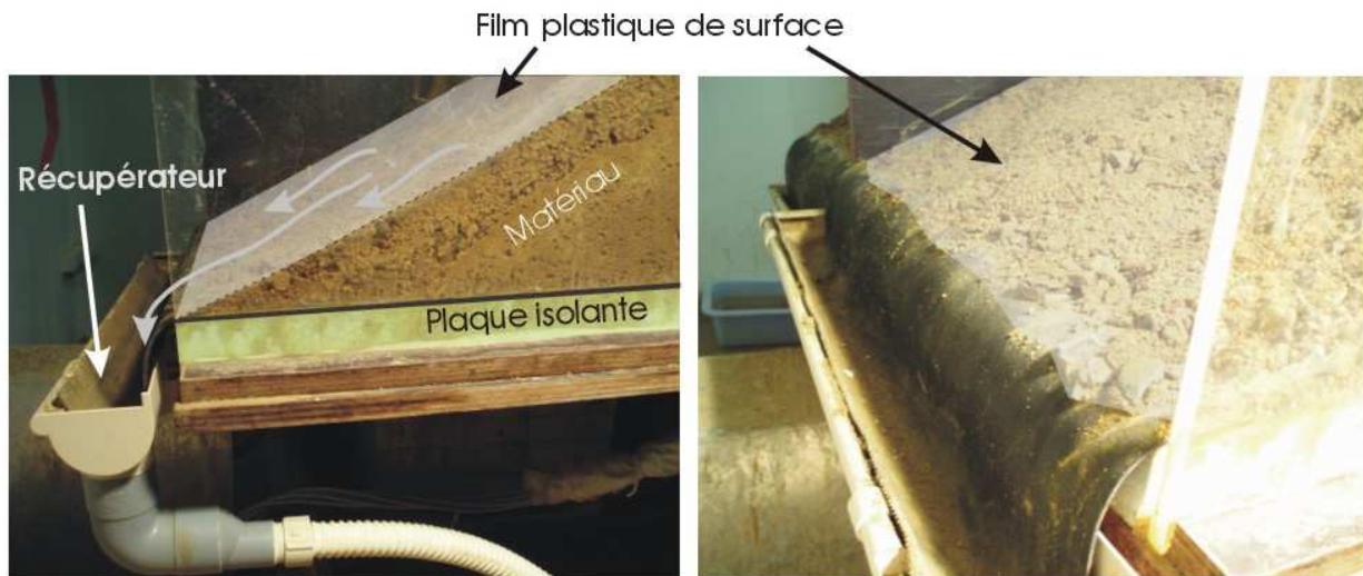
Water and eroded material recovery system.
