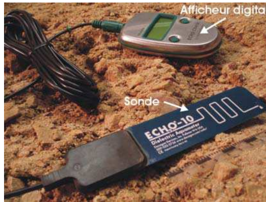
ECH2O-10 moisture content probe.
