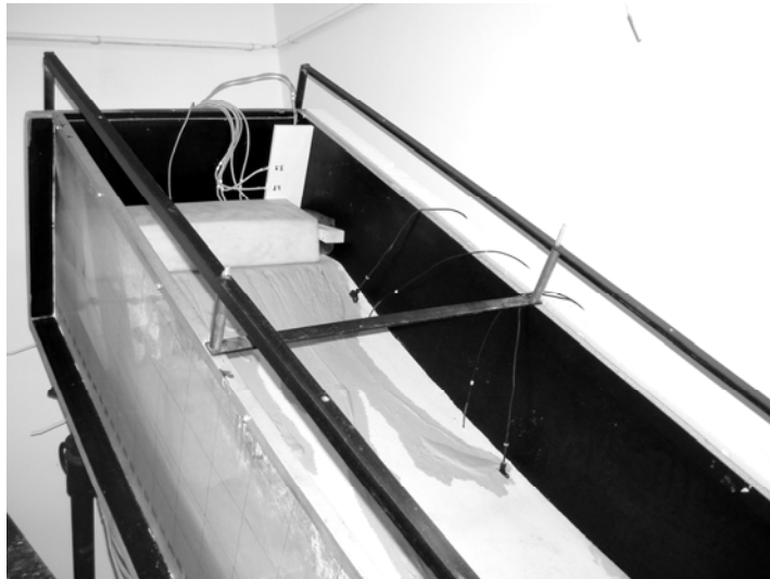
Figure 5. Close-up of the apparatus used in the physical modeling of debris flows.
