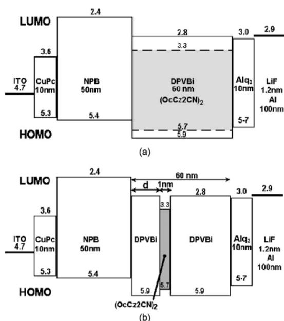
Fig. 3. Configuration of the multilayer OLEDs; (a):  $(\text{OcCz2CN})_2$ -doped DPVBi, (b): non-doped, with a 1 nm thick  $(\text{OcCz2CN})_2$  film inserted in DPVBi layer. HOMO level of  $(\text{OcCz2CN})_2$  was obtained from cyclic voltammetry. LUMO level was deduced from the optical energy band-gap  $E_g$  and HOMO values.
