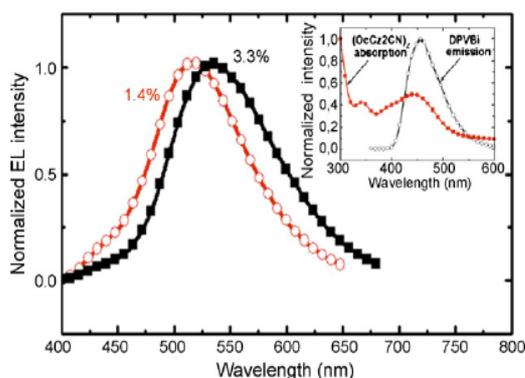
Fig. 5. Electroluminescence spectra at a current density of 10 mA/cm<sup>2</sup> of doped OLEDs with 1.4% and 3.3% wt of (OcCz2CN)<sub>2</sub> in DPVBi. Inset: proposed (OcCz2CN)<sub>2</sub> absorption and DPVBi emission spectra.
