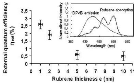
FIG. 2. External quantum efficiency  $\eta_{\text{ext}}$  (%) vs rubrene thickness in DPVBi ( $d=5$  nm) at a current density of  $30$  mA/cm $^2$ . Inset: rubrene absorption and DPVBi emission spectra.
