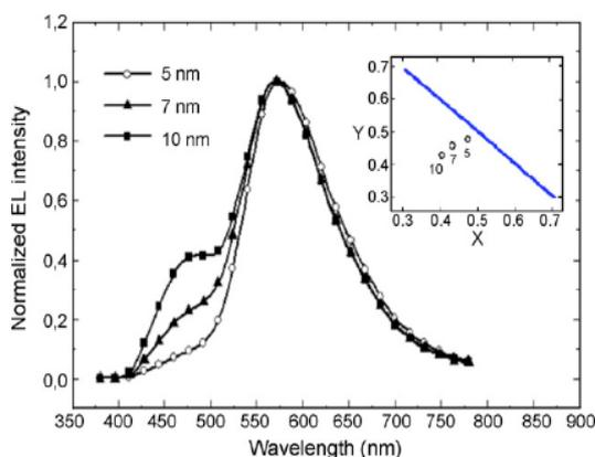
Fig. 6. EL spectra for different positions  $d$  of a 1 nm thick layer of (OcCz2CN)<sub>2</sub> from the NPB/DPVBi interface. The spectra are normalized to the yellow peak at 568 nm. Inset: corresponding CIE diagram (the solid line corresponds to the edge of the spectrum locus).
