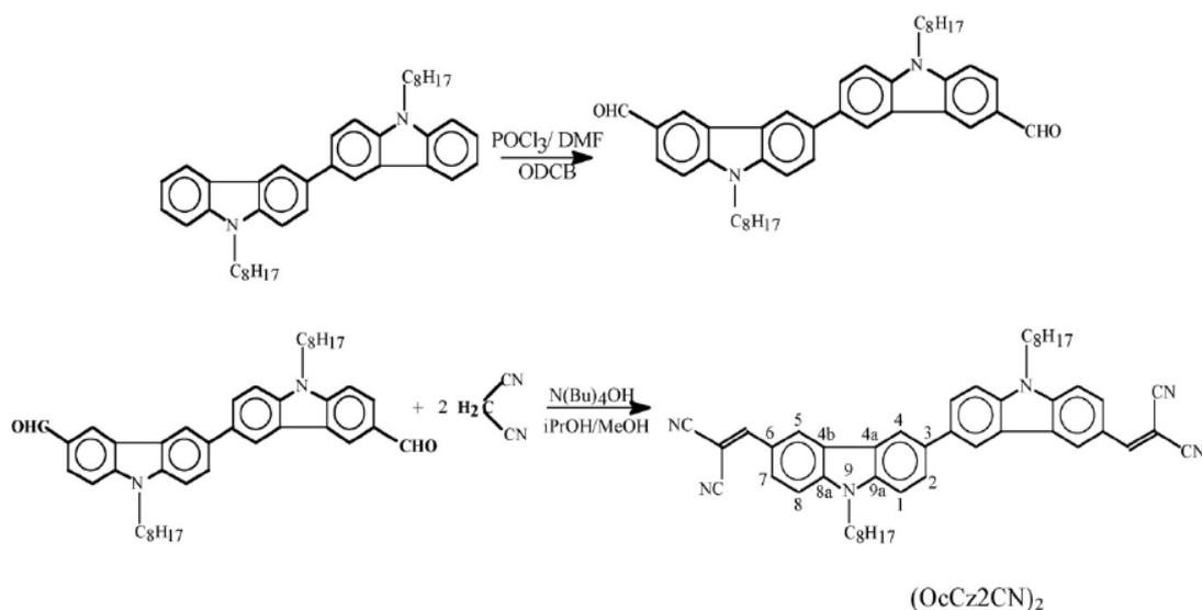
Fig. 2. Synthetic route of bicarbazylaldehyde and (OcCz2CN)<sub>2</sub>.
