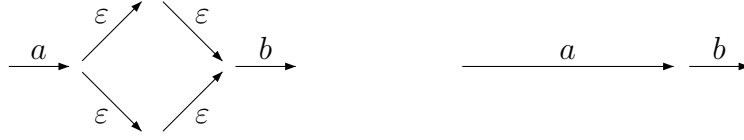
Figure 4.16: Configuration graph and deterministic transition graph of a non-deterministic terminating labeled LBM
