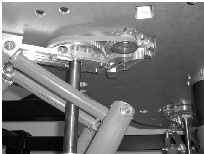
Figure 2.16. – Actuation system of each leg.
