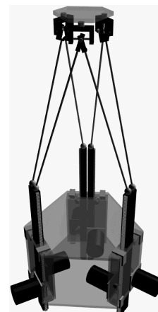
(b) Motorized manipulator for surgery. [Lazarevic 1997]
