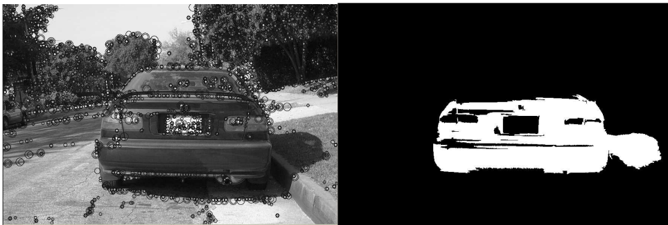
Figure 7.8: Example of SIFT features computed on an image containing a car. On the right, the associated segmented image (after region selection). The resulting mask is used to filter the key-points detected in the background: any key-point which is not in the area resulting from segmentation is not taken into account by visual detection.
