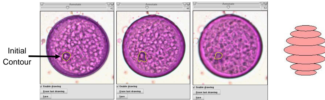
Figure 5.7: This example shows a B-snake evolving through the 2-D slices (represented on the right) of a 3-D pollen grain viewed in a light microscope. The pori (subpart of the grain) has been initially segmented by using the intelligent scissors. The initial contour is then automatically propagated through slices by adapting itself to the pori morphology.
