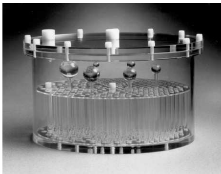
Figure 8.16: Phantom device used to simulate moving spheres during data acquisition.
