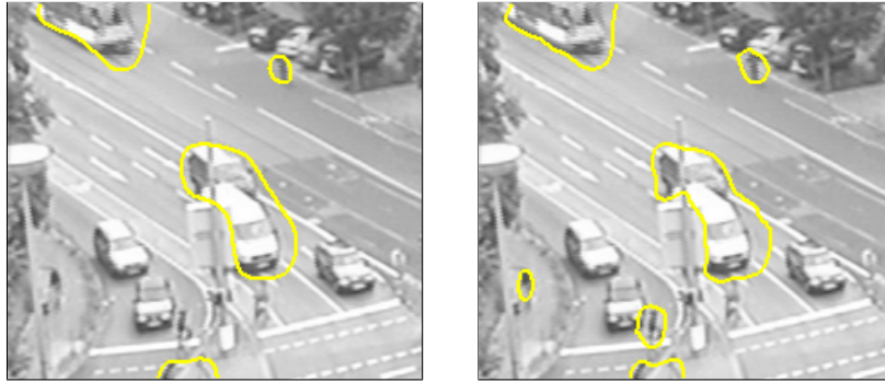
Figure 3.23: Detection of moving objects between frame 130 and 131 in the stau2 sequence. LEFT: Using optical flow. RIGHT: Using intensity, optical flow, and texture.
