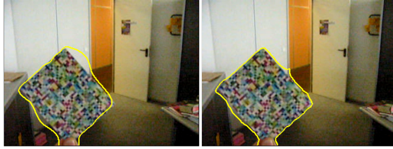
Figure 3.25: Object detection in the box sequence. LEFT: Using optical flow. RIGHT: Using color, optical flow, and texture.
