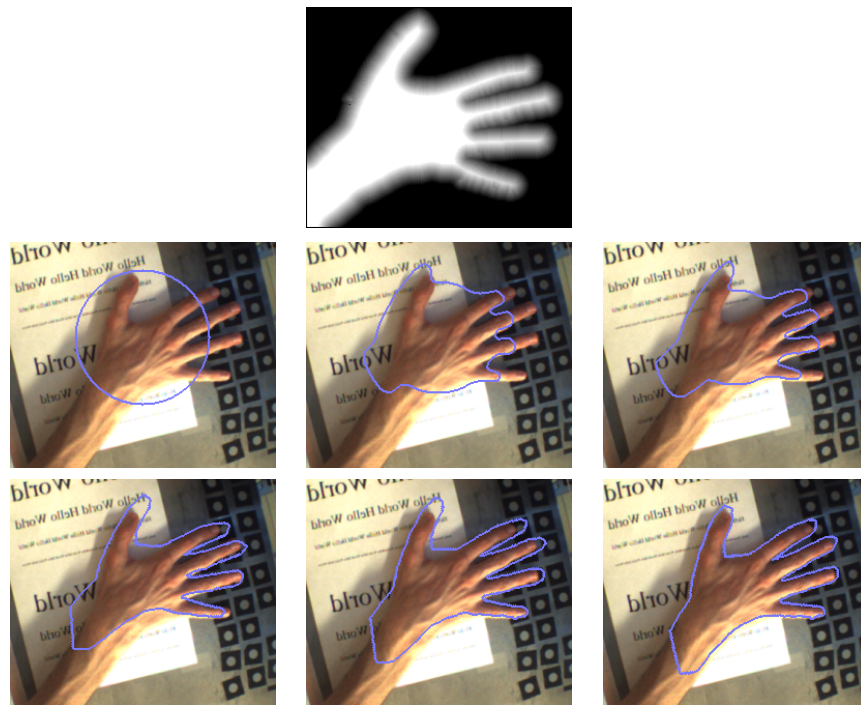
Figure 4.23: Constrained segmentation with a single static prior - TOP: Hand shape prior, BOTTOM: Constrained curve evolution.
