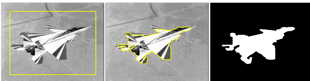
Figure 2.13: F15 image - Contour initialization and final segmentation using Parzen density estimates ( \sigma = 20 ).
