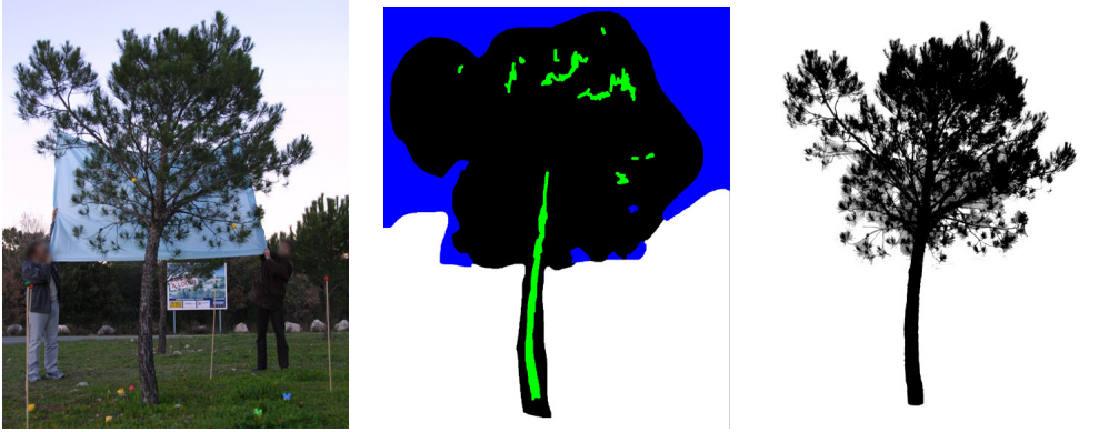
Figure 4.4: Left: the original image. Middle: the regions specified roughly by the user as foreground and background. Right: the computed alpha-mask (note that we used black for opaque for clarity of the figure).
