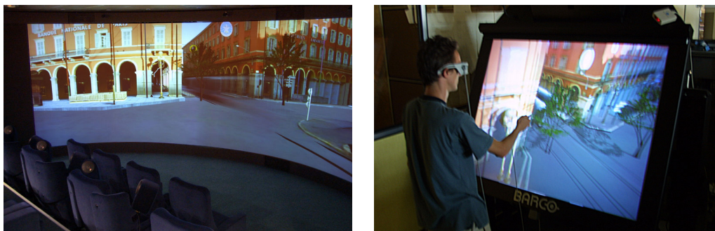
Figure 5.8: The VE of the urban planning/architecture application as displayed on an immersive curved-screen display and on a workbench.
