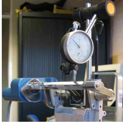
Figure 4.4. A 0.01mm resolution dial gauge was used to measure the mechanical backlash, stiffness, and positioning reproducibility of the robot prototype.
