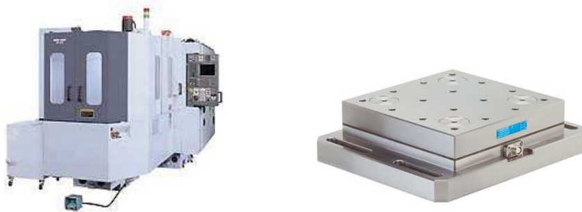
Figure 3.3. Industrial Milling machine (left) and force sensor (right) used for the milling experiments [Photos taken from Mori Seiki and Kistler websites, respectively].
