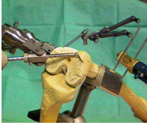
Figure 5.15 Preliminary milling experiments using a custom built milling tool on synthetic bones.
