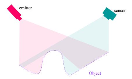
Figure 5: One of acquisition problem: hiding area. The visibility area of the emitter (pink) and the sensor/receiver (green). Some surface regions may be visible from the emitter and not visible from the receiver and vice versa.
