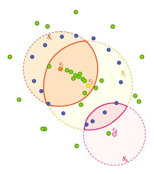
Figure 7.5: Input points (blue) and centers (green). The support of  $\phi_i$  and  $\phi_j$  ( $S_i$  and  $S_j$ ) intersect and share several centers so  $a_{i,j} \neq 0$ . The support of  $\phi_i$  and  $\phi_k$  ( $S_i$  and  $S_k$ ) does not intersect so  $a_{i,k} = 0$ .
