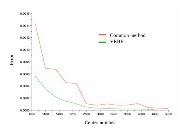
Figure 8.6: Plot of the error against the number of centers (from 1K and 5K) for the Dinosaur model (15k input points). The red curve corresponds to the common method. The green curve corresponds to our approach (with filtering and clustering).
