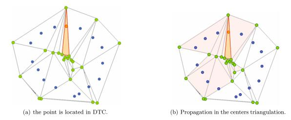
Figure 7.7: Dual method. Input points (red), the centers (black) and the Delaunay triangulation of centers (gray).
