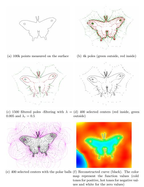
Figure 8.2: Algorithm sequence in 2D with filtering and clustering.
