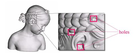
Figure 6: Reconstructing the Bimba con nastrino. The registration and fusion stages have been made with Minolta's software). Some holes appear (right) where the scan can not capture the shape (deep area)
