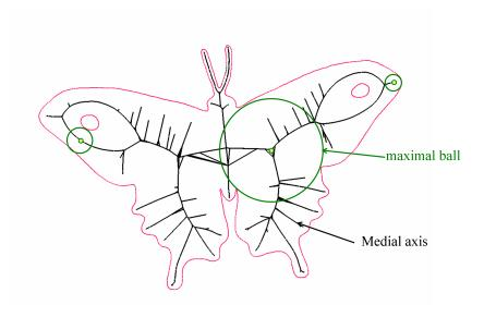
Figure 4: Inside Medial Axis. A 2D shape (red) and its inside medial axis (black).
