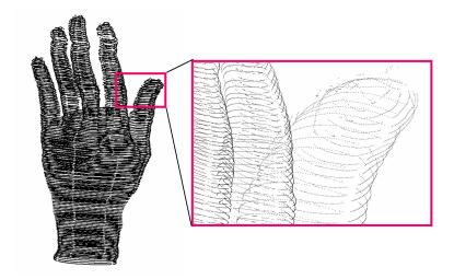
Figure 8.13: Noisy hand model (90K input points). The input points result from registering three range maps.
