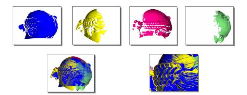
Figure 4: Registration. Top: Four range images of the Bimba con nastrino (18 range images were necessary to scan the sculpture). Bottom left: the range images are merged. Bottom right: detail of the braid.
