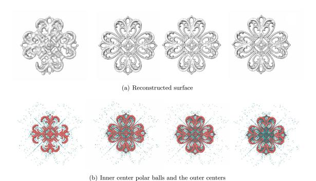
Figure 8.16: Effect of the greedy selection on the Filgree model (80K input points). The number of centers is form the left to the right 5K, 10K, 15 and 18K. The overlapping rate threshold is  $\rho = 0.6$
