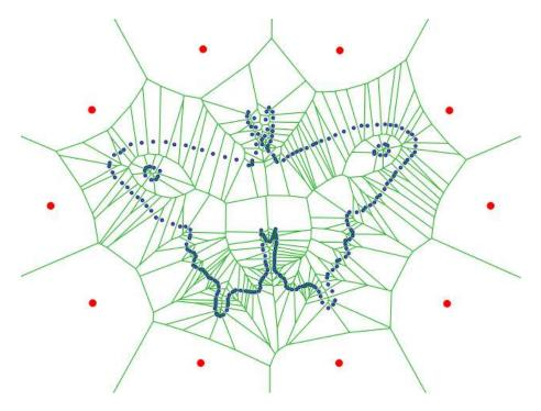
Figure 7.2: The Voronoi diagram of the input points set augmented by the bounding box points (red points)
