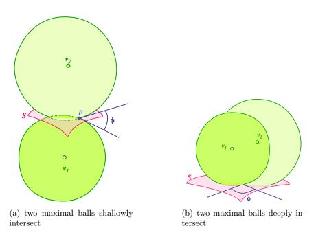
Figure 7.4: The two cases of maximal ball intersection. Left: when the two poles are on each side of the surface. Right: when the two poles are on the same side of the surface.
