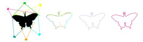
Figure 3: Scanning pipeline. Left to right: Acquisition (the physical object is acquired by several scanning process in order to cover all the surface), registration and merging.
