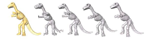
Figure 8.7: Reconstruction sequence of the Dinosaur with increasing number of centers. From left to right: original, then reconstruction with 1K, 3K, 4K and 5K centers.
