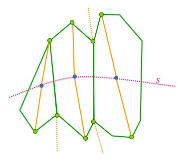
Figure 7.3: Edges of the poles graph in 2D. There are two king of edges joining two poles. Orange edges when the 2 poles share a vertex (case 1) and Green edges, Voronoi edges, when the poles are neighboor in the Voronoi diagram (case 2)
