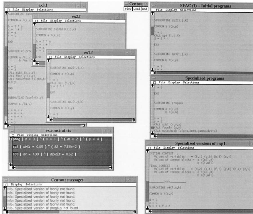
Figure 19. Partial evaluation of a Fortran 90 application (with reuse of specialized versions).
