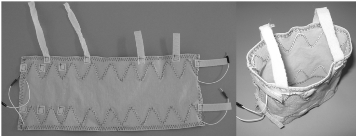
Fig. 1. The inductance plethysmographic jacket adapted for preterm neonates. Only horizontal wiredrawing is possible. Lateral bands permit to adapt the jacket size to the neonate's body.
