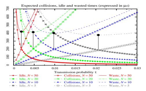
FIG. 6.2 – Expected wasted time, expected time spent in collisions and expected idle time in a virtual transmission time for different values of N ( $T_c = 4335 \mu s$  and  $\sigma = 20 \mu s$ ).
