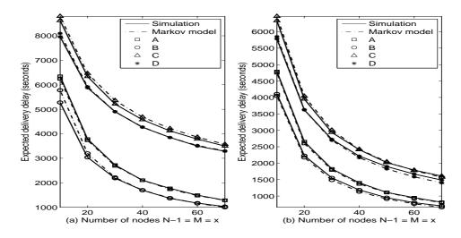
FIG. 3.7 –  $\mathbf{E}[T_{MTR}](\mathbf{a})$  and  $\mathbf{E}[T_{ER}](\mathbf{b})$ : (A) Throwboxes are connected and uniformly distributed, (B) Throwboxes are connected and stationary distributed, (C) Throwboxes are disconnected and uniformly distributed, (D) Throwboxes are disconnected and stationary distributed.
