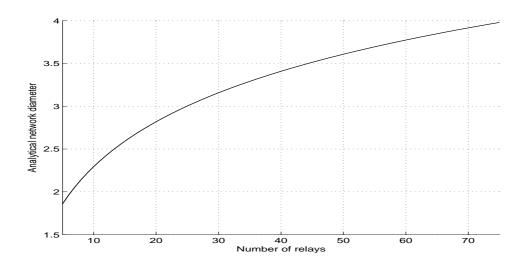
FIG. 5.2 – Analytical network diameter plotted versus the number of relays.
