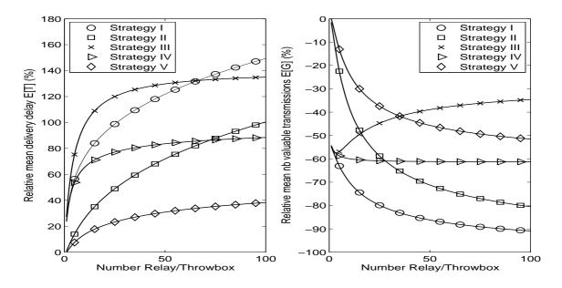
FIG. 4.2 – Relative mean delivery delay  $\mathbf{E}[T]$  (left) and relative mean number of transmissions  $\mathbf{E}[G]$  (right) obtained under each strategy with respect to epidemic protocol.
