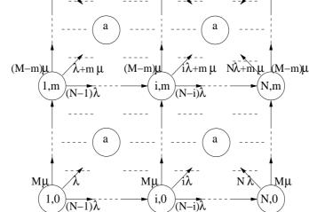
FIG. 3.1 – Transition rate diagram of the Markov chain in the case of MTR protocol and disconnected throwboxes.
