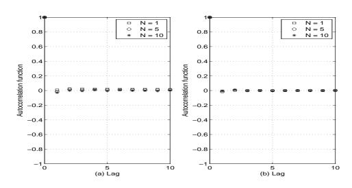
FIG. 2.3 – Autocorrelation function of inter-meeting times over 10 lags between N throwboxes and a mobile node moving according to the RWP model (a) and the RD model with reflection (b).
