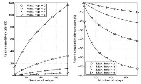
FIG. 5.3 – Relative mean delivery delay (on the left) and number of copy transmissions (on the right) with respect to epidemic protocol versus the number of relays.
