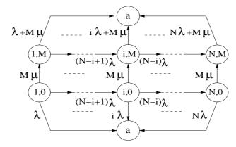
FIG. 3.2 – Transition rate diagram of the Markov chain in the case of MTR protocol and connected throwboxes.
