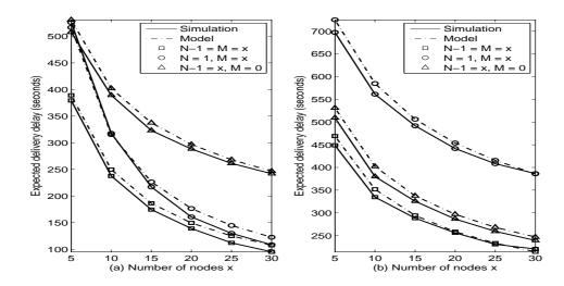
FIG. 3.3 –  $\mathbf{E}[T_{MTR}]$ : (a) Throwboxes are connected, (b) Throwboxes are disconnected.
