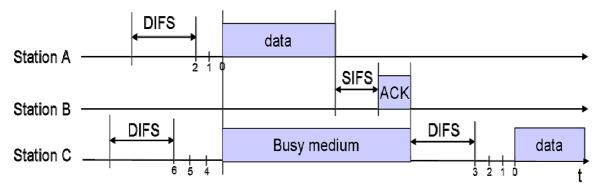
FIG. 6.11 – Basic access DCF mechanism.
