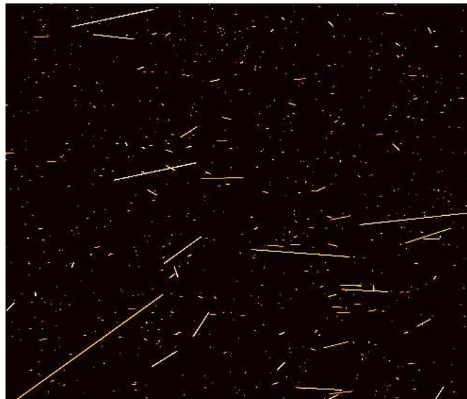
Figure 7.20: An example of FOV dominated by PPEs with a fluence of 100 particles/cm 2 /s. As no stars are visible on this snapshot, all objects are discarded as PPEs.
