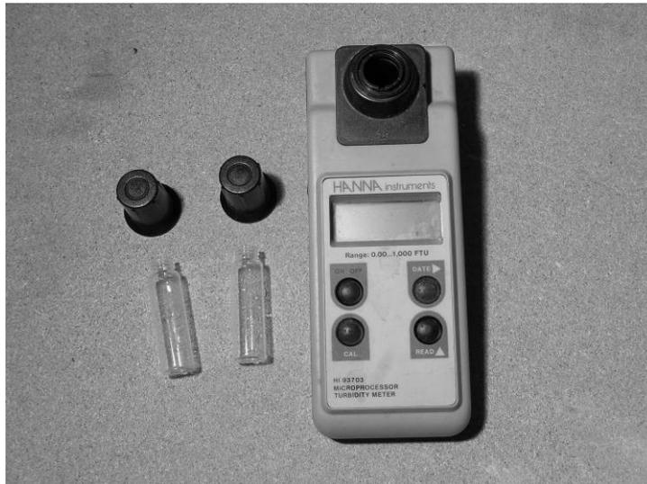
Figure 3.4 Turbidity measurement apparatus.
