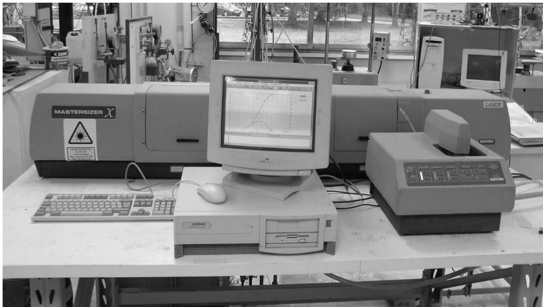
Figure 3.7 The laser granulometer.
