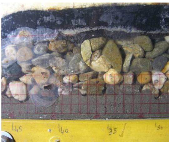
(e)  $v = 2.59$  cm/s (Failure erosion)
