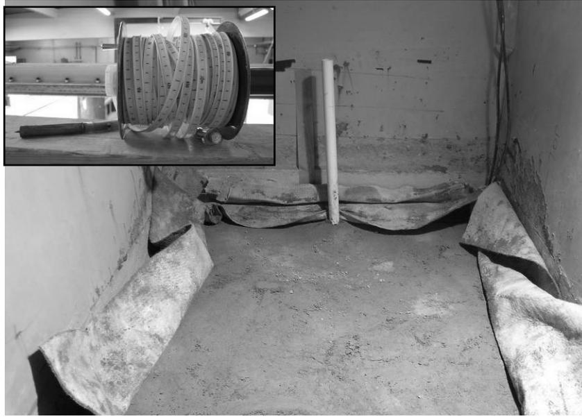
Figure 3.6 Water level observation well and indicator.
