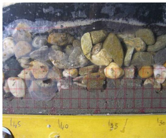
(f)  $v = 2.88$  cm/s (Failure erosion)
