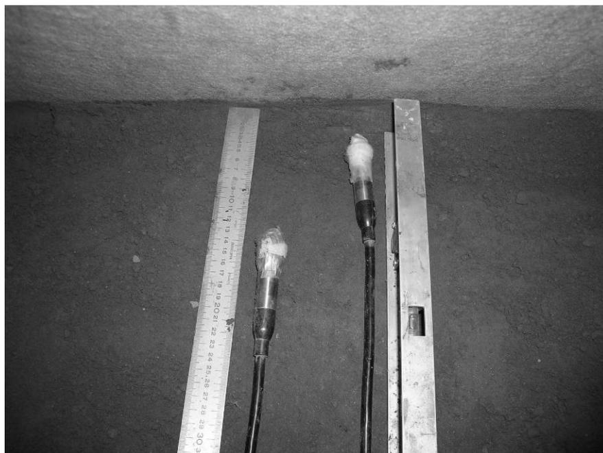
Figure 3.5 Water pressure monitor - piezometers.
