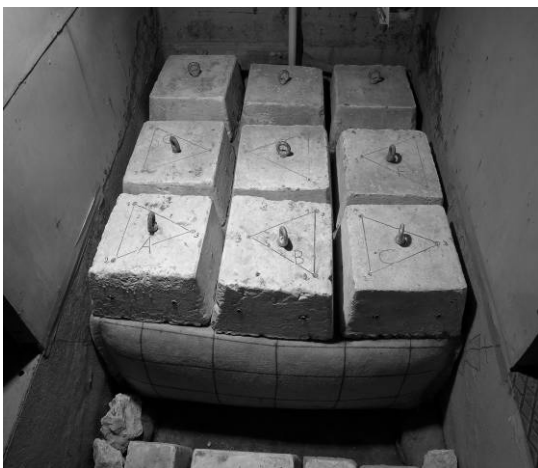
(e) Place the concrete blocks.
