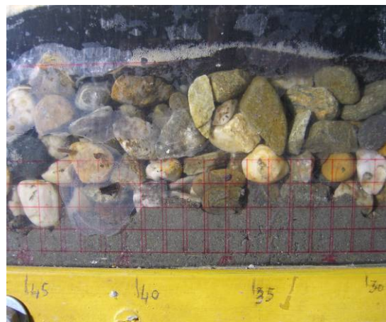
(f) v = 2.88 cm/s (Failure erosion)
