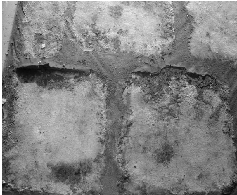
Figure 3.34 The eroded particles deposited on the surface of geotextile (Test 3).
