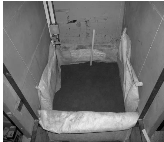
(b) Fill and compact soil by layers.
