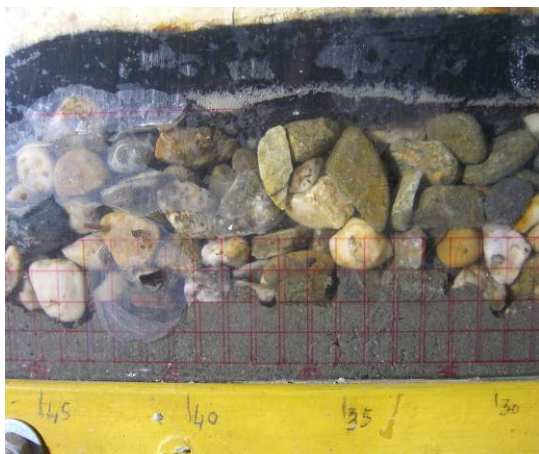
(e) v = 2.59 cm/s (Failure erosion)
