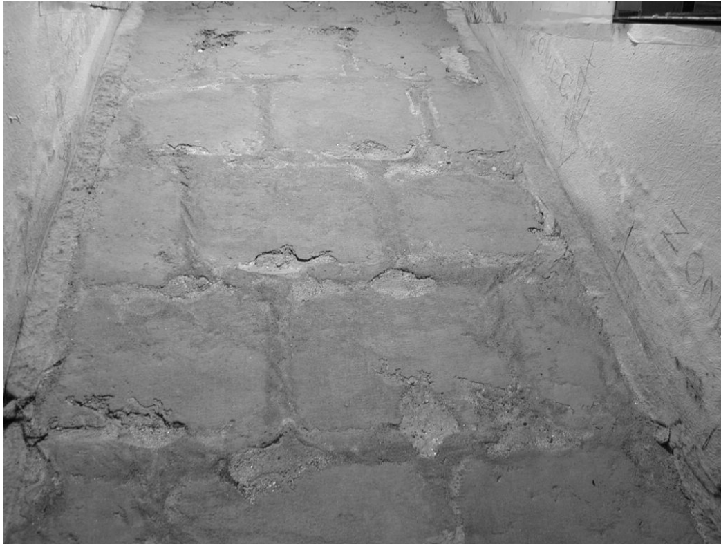
Figure 3.35 The eroded particles deposited on the surface of geotextile (Test 3).
