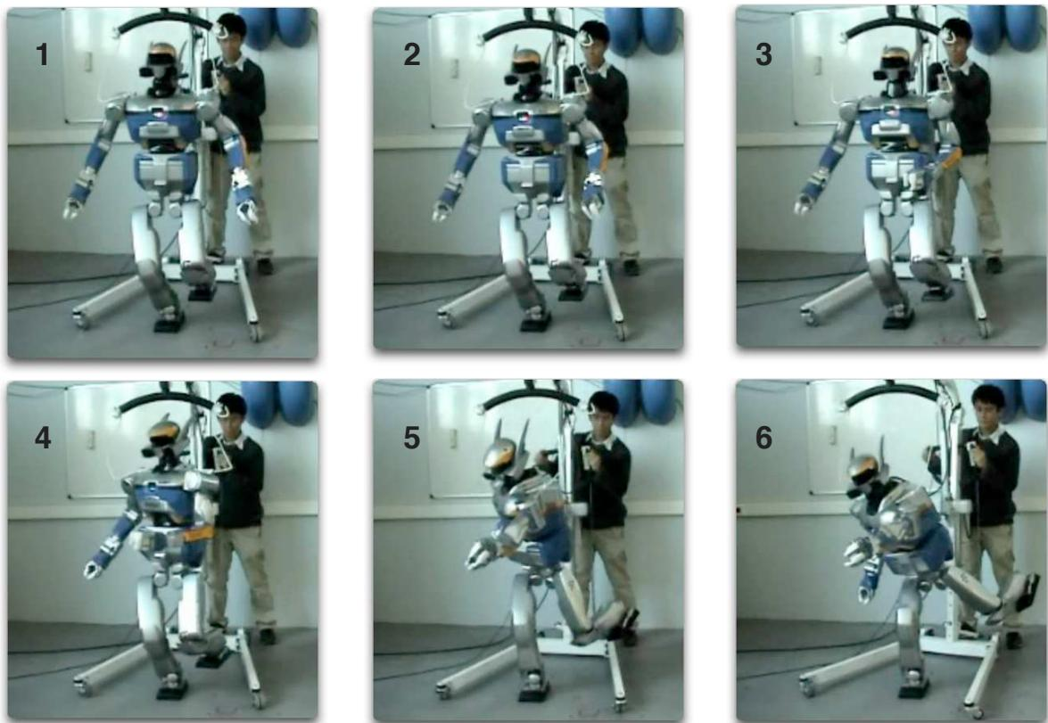
**Figure 9.4:** Snapshots of the whole body reaching motion
