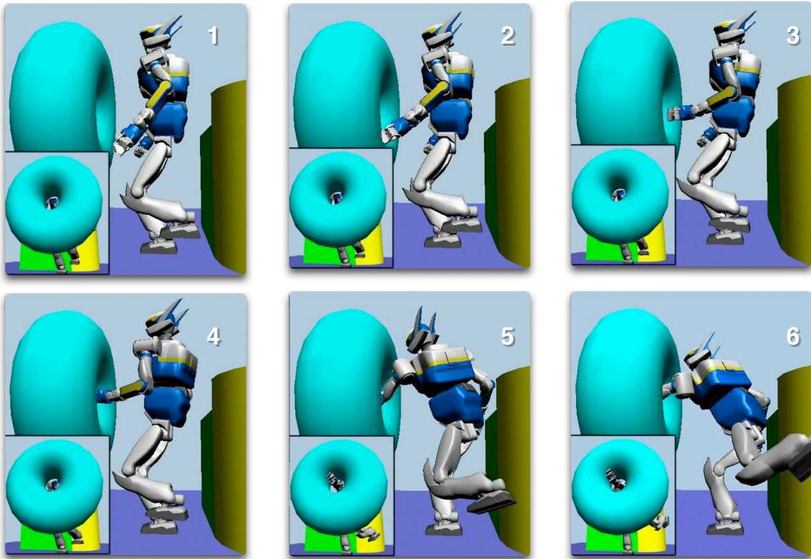
**Figure 9.1:** Whole body reaching with collision avoidance
