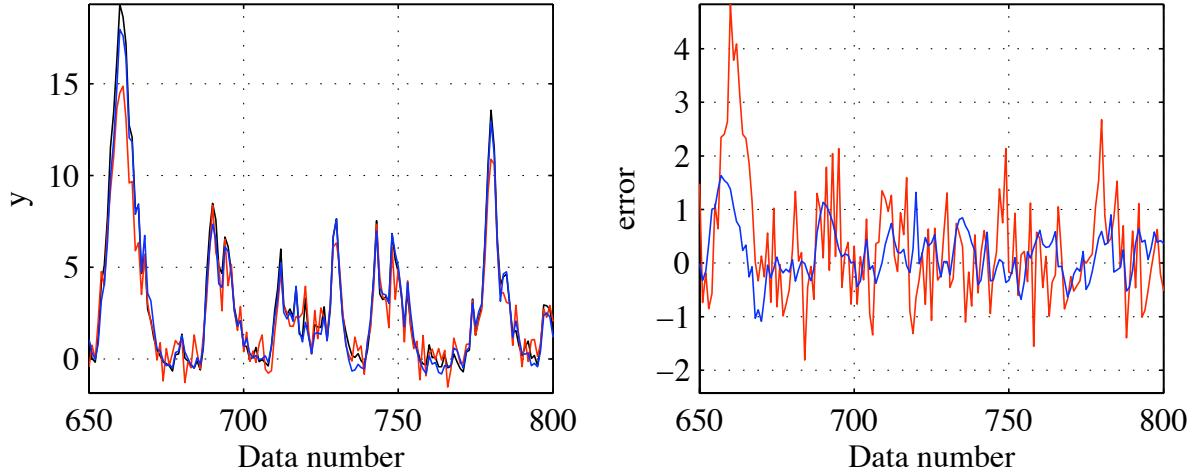
(a) The real output *without* the measurement noise (black line). The outputs of quadratic system (blue line) and NNOE model (red line), and their errors.
