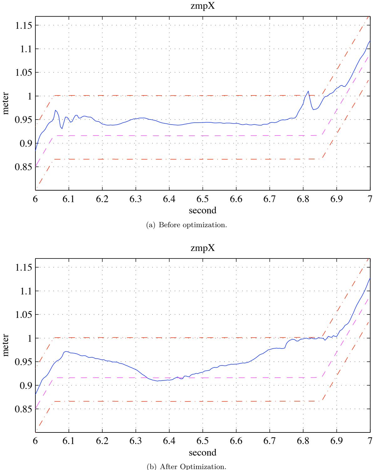
**Figure 7.6:**  $x$  coordinate of ZMP: the solid blue line is the measured  $ZMP_x$ , the red dash-dotted lines design the safe stability zone and the magenta dashed line denotes the designed reference. The oscillations around 6.1 and 6.8 seconds disappear after optimization as well as the surge at 6.81 second.
