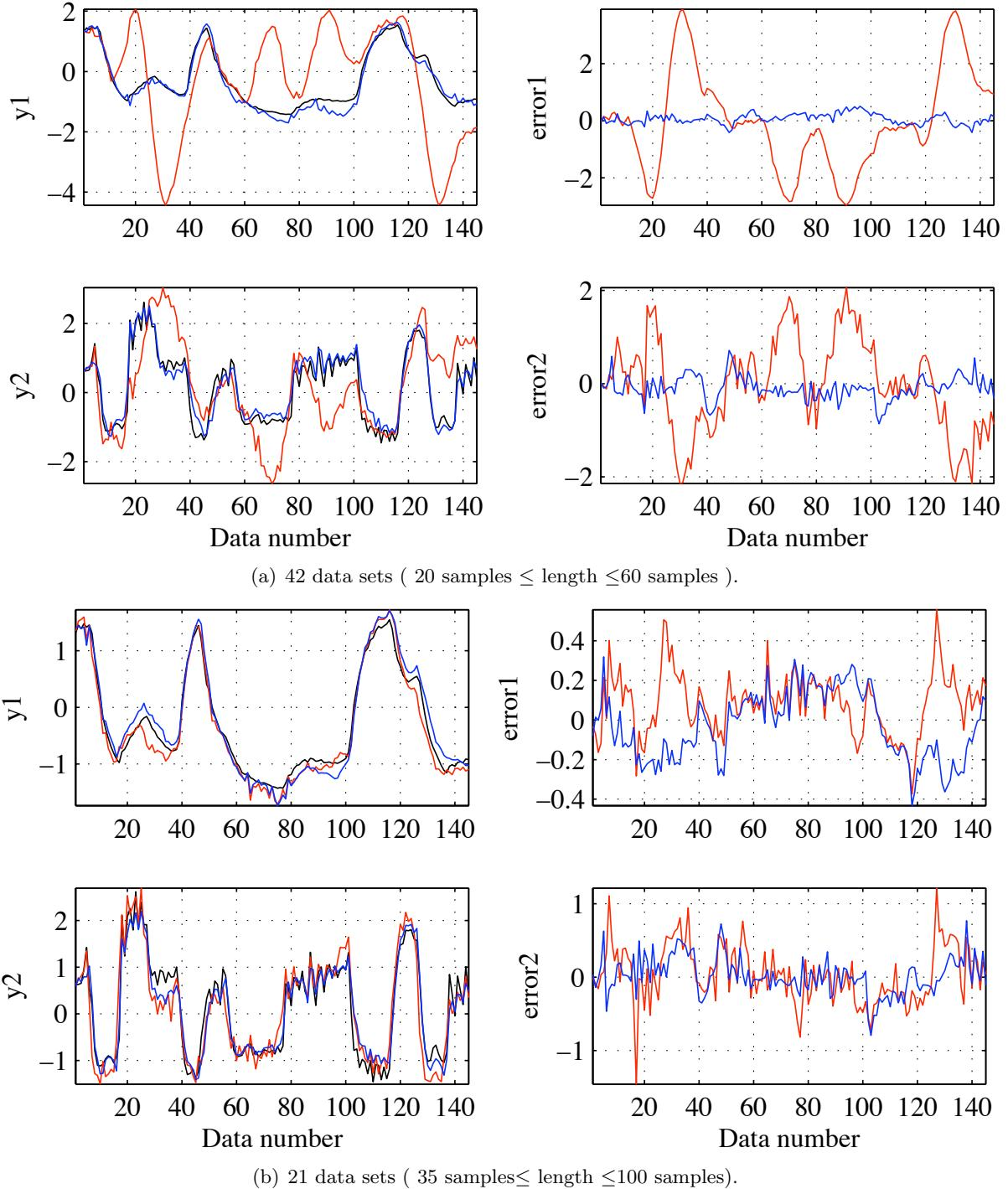
**Figure 3.8:** The output of industrial winding process (black line), and the outputs of the linear model obtained by our method (blue line) and N4SID method (red line) are superimposed.
