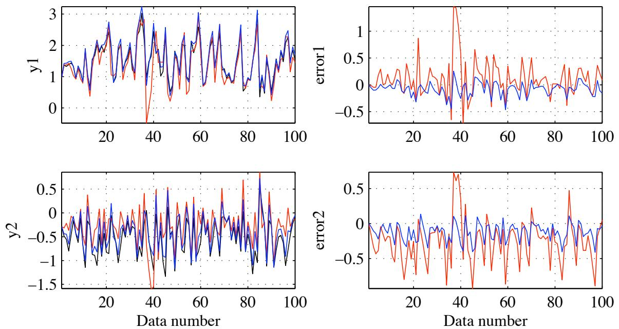
**Figure 5.3:** The real outputs of QSS *without noise* (black line). The outputs of the identified QSS using all data sets (blue line) and the identified QSS using a single data set (red line) and their errors are superimposed.
