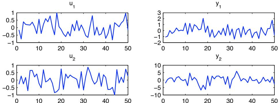
**Figure 3.2:** The inputs  $u_1$  and  $u_2$  are sum of sinusoidal signals, and the outputs are  $y_1$  and  $y_2$ .
