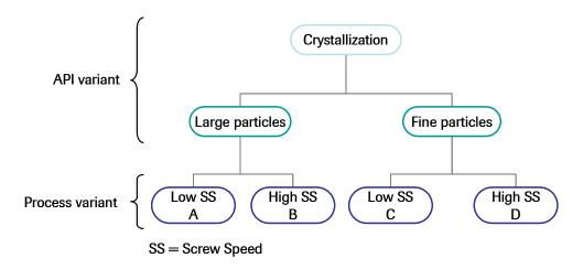
Figure 27. Process variants and corresponding batches. One API variant: the particle size and one process variant: the screw speed were under investigation. Four batches, A, B, C, D were then analyzed by NIR-CI.
