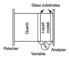
Figure 9. Schematic view of a Lyot filter element
