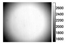
Figure 7. Spatial instrument response curve (median values computed over wavelengths) registered using a high reflectance standard. Non-uniform illumination of the detector due to the optics of the camera is depicted.
