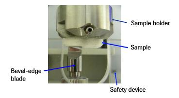
Figure 23. Instrumentation used in the laboratory to flatten the analysis surface of the tablets
