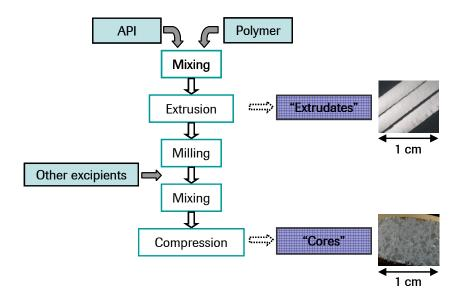
Figure 26. The process workflow employed to produce the tablets. It was constituted of five main steps. The two process intermediates which were studied were the extrudates (top right picture) and the cores (bottom right picture).
