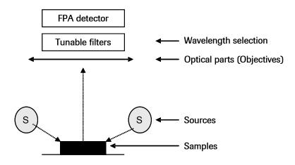
Figure 8. Schematic view of a NIR spectrometer using tunable filter. Adapted from [16].
