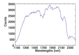
Figure 10. Spectral instrument response curve (median values computed over pixels) registered using a high standard reflectance.
