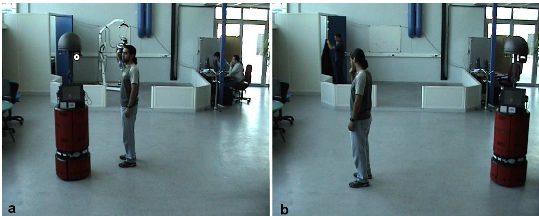
Figure 5.14: The effect of the Visibility Criterion (§ 3.4) for a path passing in front or behind of a person.
