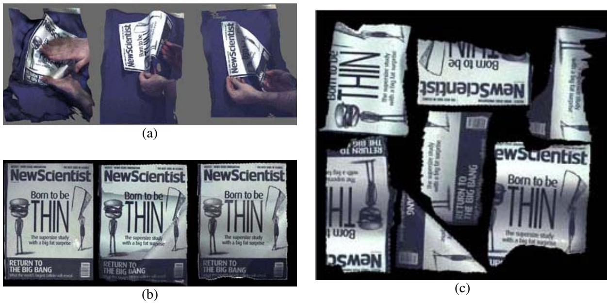
Figure 7.5: Paper (BMVA-Symposium'08) – Automatic Quasi-Isometric Surface Recovery and Registration from 4D Range Data . (a) shows some inputs range images, (b) shows detected isometric patches that were flattened and (c) compares the true surface texture (left), the rigidly registered patches (middle) and the non-rigidly aligned patches (right).
