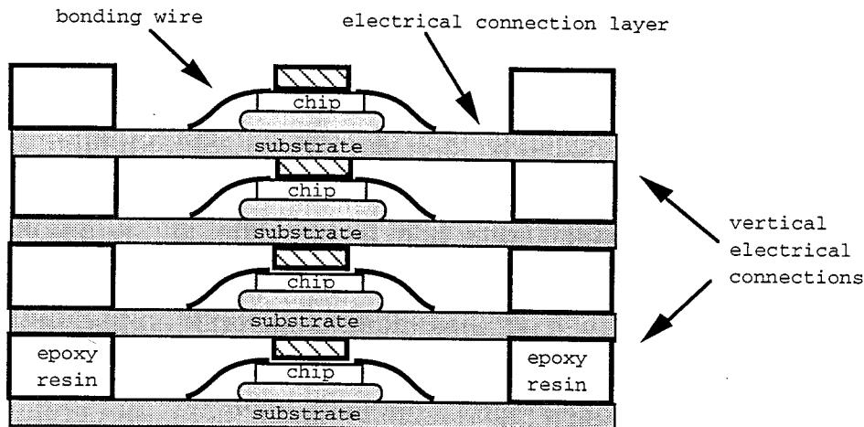
*Fig. 4.2.1.1.1. Integrating different chips into one package using the MCM-V technique*
