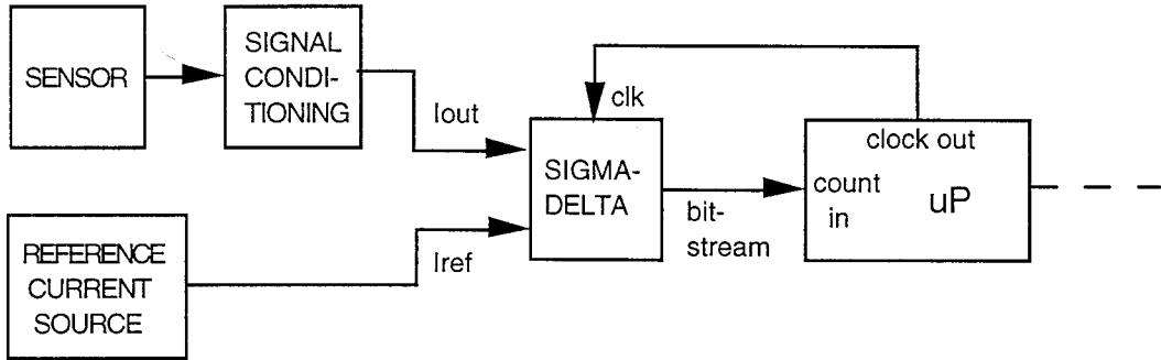
*Fig. 4.2.2.2.1. One-sensor measurement configuration using a sigma-delta bitstream converter*
