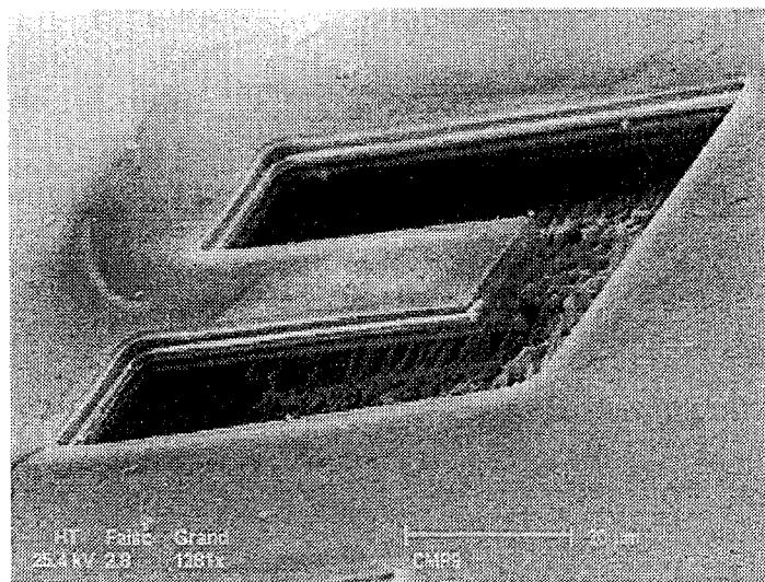
*Fig. 2.3.2.3.2.2. Structure manufactured using 0.6 $\mu$  GaAs MESFET compatible front-side bulk micromachining*
