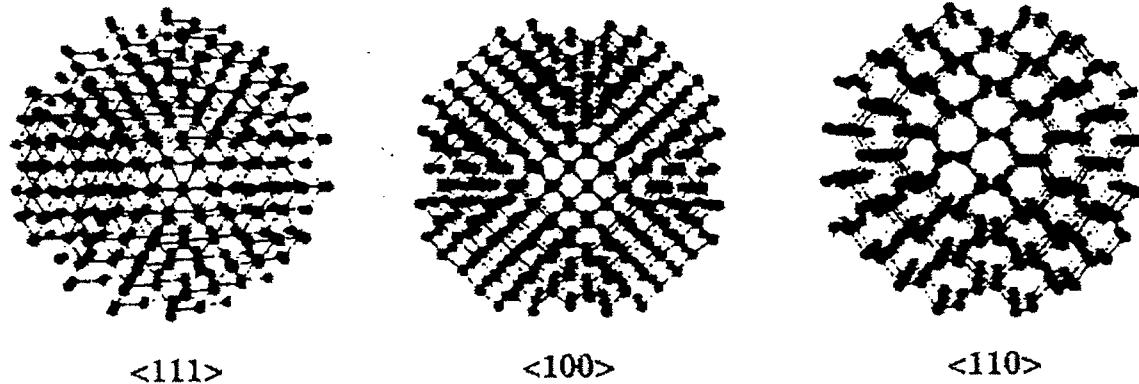
*Fig. 2.2.3.1.1. Orthogonal view through the main planes of the silicon crystal*
