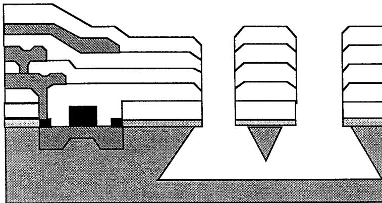
*Fig. 2.3.2.3.2.1. Cross-sectional view of a microbridge with a MESFET using the Vitesse process*
