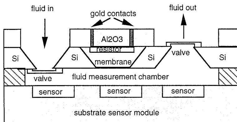
*Fig. 4.2.1.2.1. Cross section of the micropump module and the sensor module*
