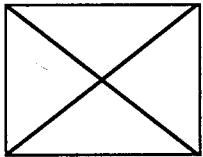
Fig. 2.2.3.2.1.1. Pyramid formed in the silicon etched through a rectangular mask.
