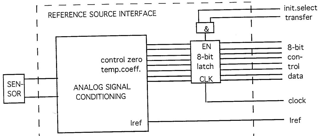
Fig. 4.3.3.4.1. Interface module for the BARMINT reference source
