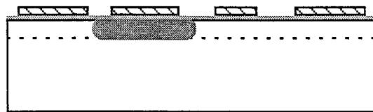
Step 8 : - Photoresist elimination
