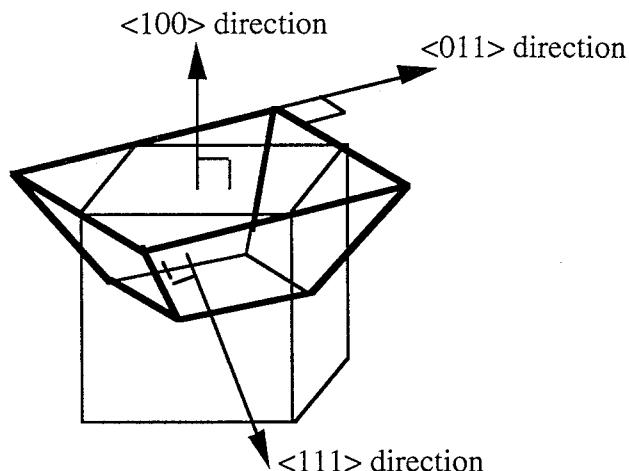
*Fig. 2.2.3.1.2. Microscopic consideration of the etching.*
