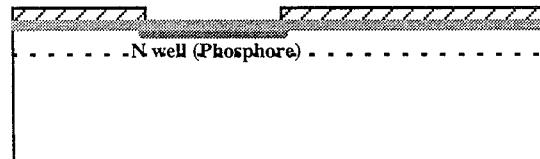
**Step 5 : - Photoresist elimination**
