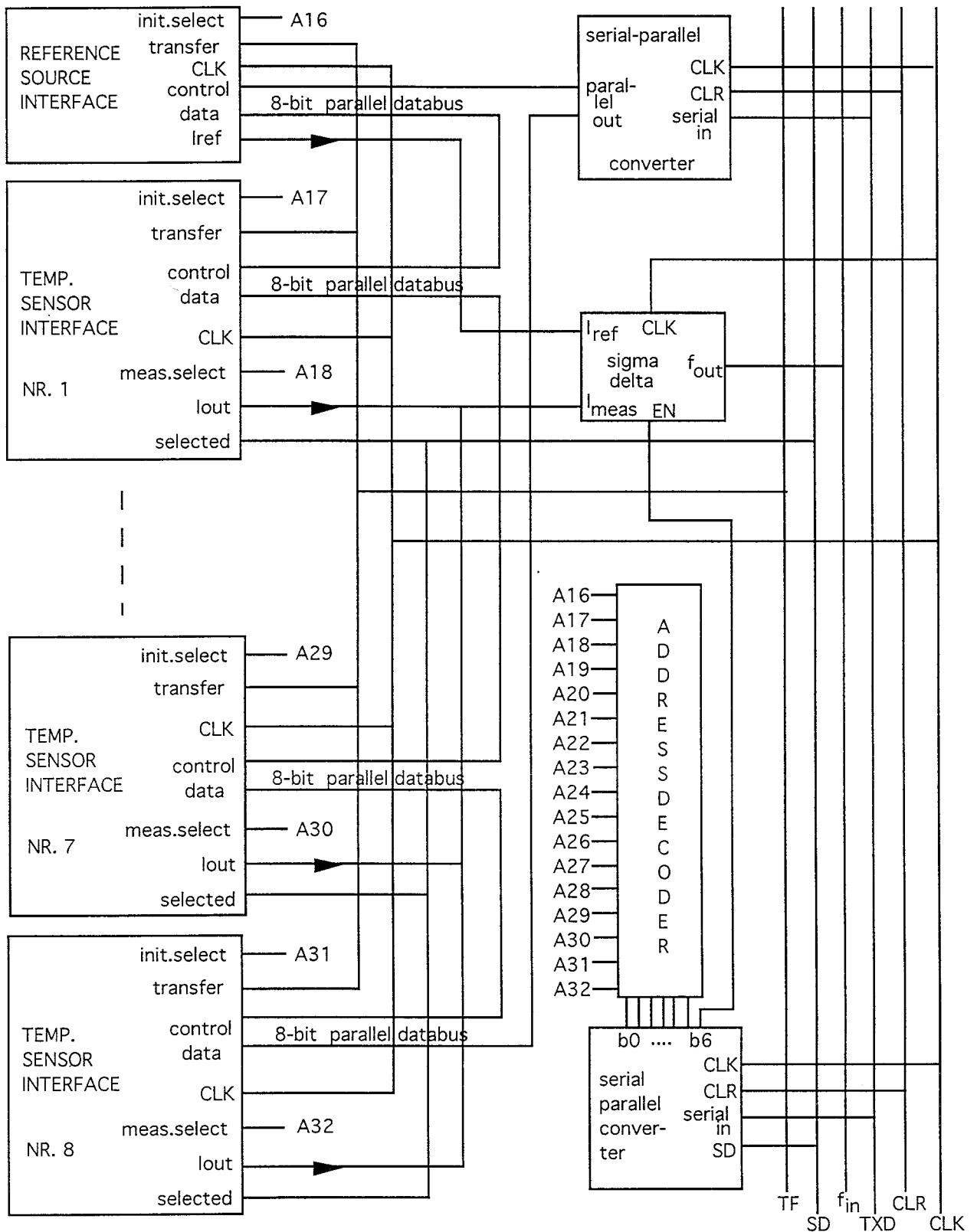
Fig. 4.3.4.1.2. System level configuration of the BARMINT VLSI module
