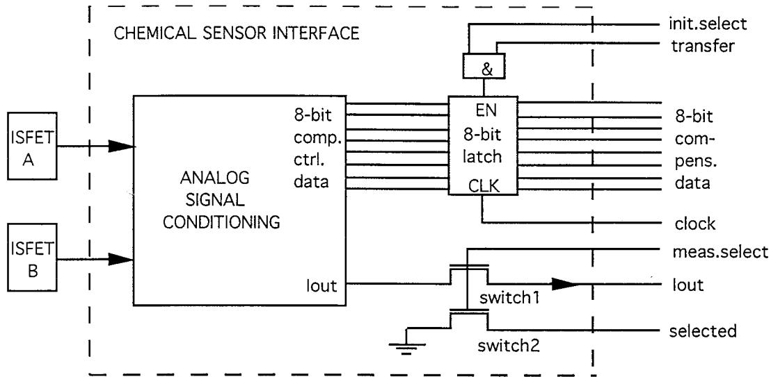
Fig. 4.3.3.6.1. Chemical sensor interface module for the BARMINT microsystem
