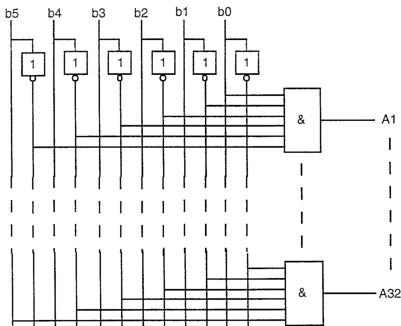
Fig. 4.3.4.5.1. Principle of the address decoder for the BARMINT microsystem.
