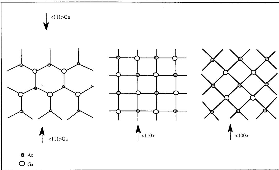
*Fig. 2.3.2.2.1.1. Schematic projections of the atoms in the three low-index planes of GaAs*
