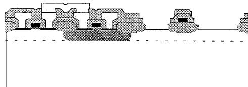
Step 16 : Passivation layer deposition
