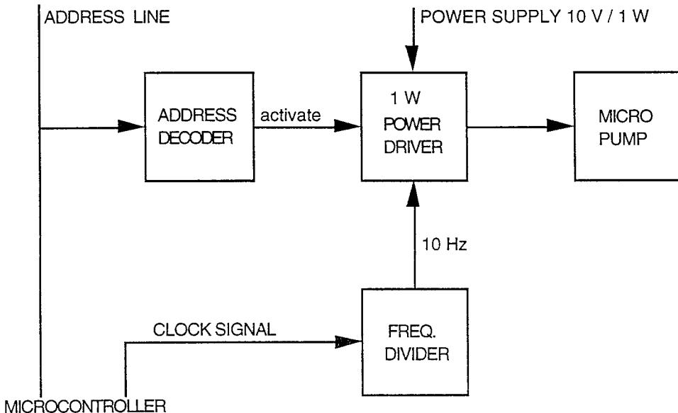
Fig. 4.2.2.4.1. The actuator control configuration for the BARMINT microsystem
