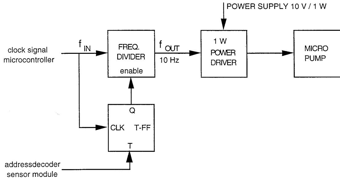
*Fig. 4.3.4.2.1. Optimized control configuration for the BARMINT micropump*
