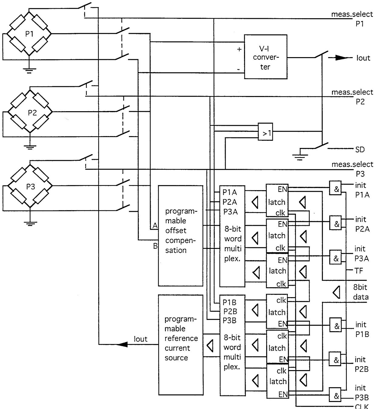
*Fig. 4.3.3.5.1. The configuration of the BARMINT pressure sensor interface module*
