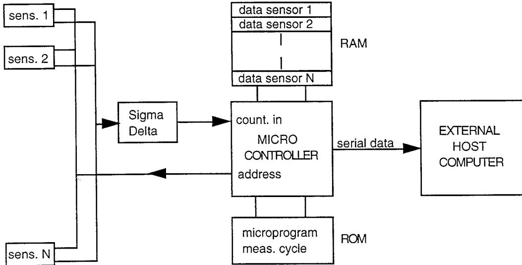
Fig. 4.3.1.3.1. The sensor measuring cycle proposed for the BARMINT microsystem
