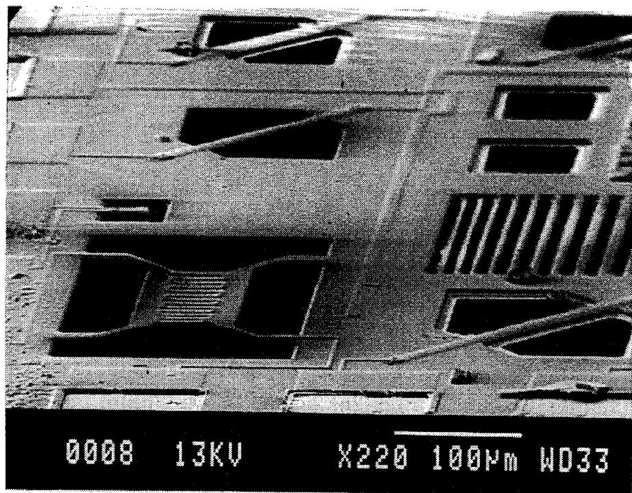
Fig. 2.2.3.3.2.1. SEM photograph of the main structures fabricated monolithically with ICs using front-side CMOS bulk micromachining
