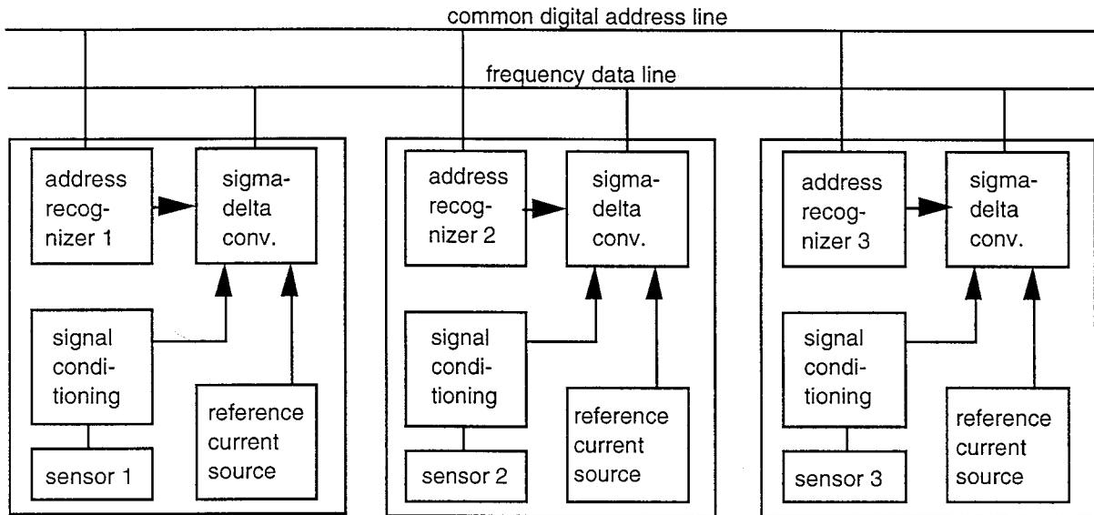
*Fig. 4.2.2.3.1. Semi-digital bus structure for internal communication in a microsystem*
