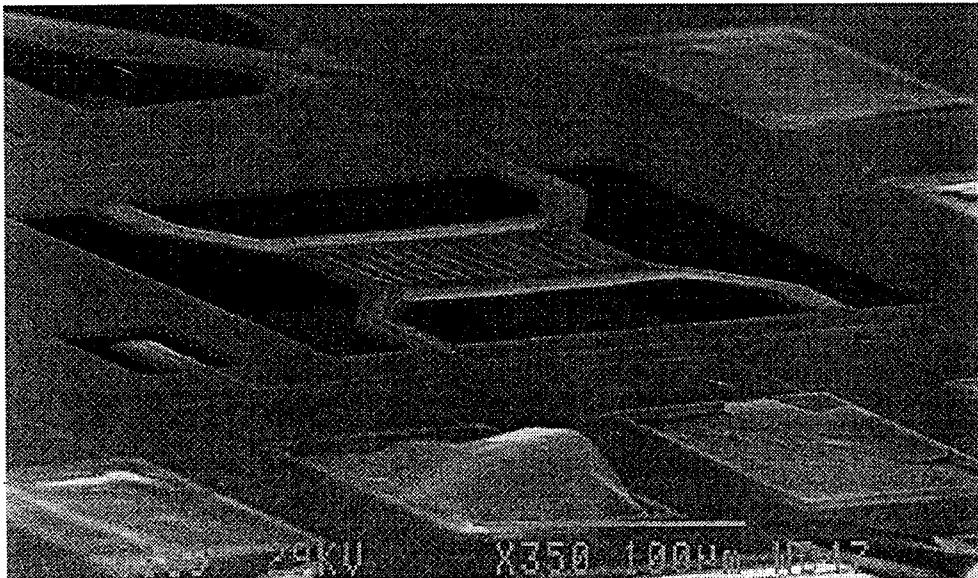
Fig. 2.2.3.3.2.3. SEM photograph of different structures etched by TMAH (the pads have suffered from the attack)
