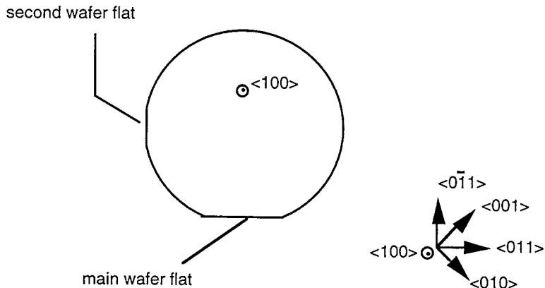
*Fig. 2.2.1.3. (100) P-type silicon wafer and its wafer flats*
