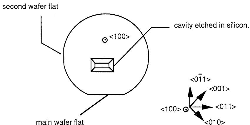
Fig. 2.2.3.2.1.3. Cavity alignment with the wafer flats.
