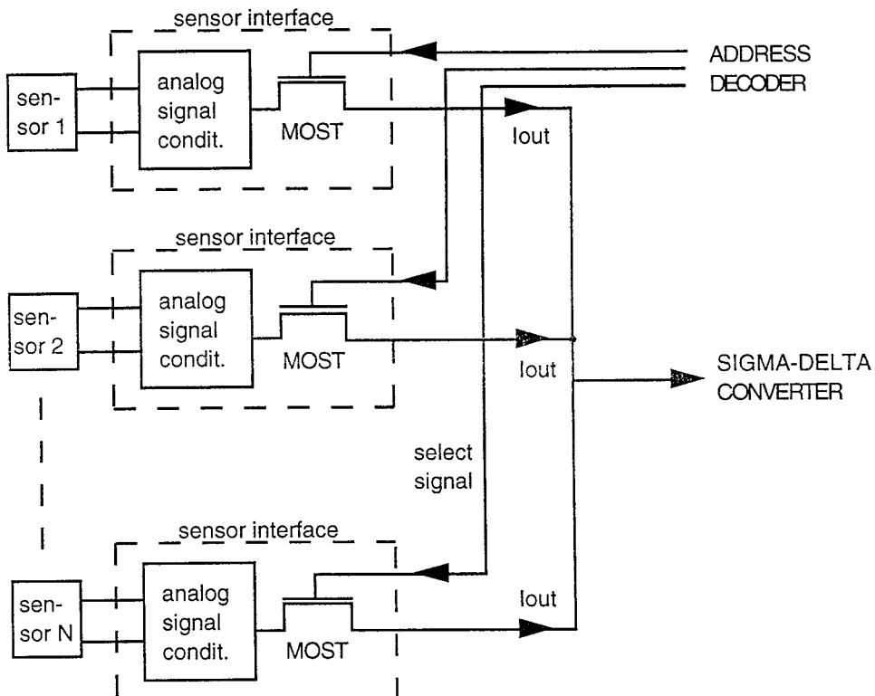
Fig. 4.3.3.2.1. Merging addressable current switches with sensor interface modules
