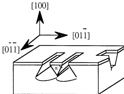
Fig. 2.3.2.2.3.1. Etched profiles in (100) GaAs by the  $\text{Br}_2\text{CH}_3\text{OH}$ -system.
