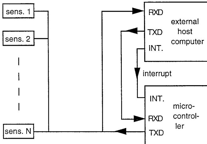
*Fig. 4.3.4.3.1. Bidirectional communication with external host computer*
