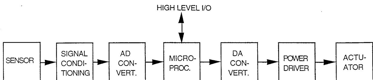
*Fig. 4.2.2.2. Basic configuration for a modern sensing and actuating system*
