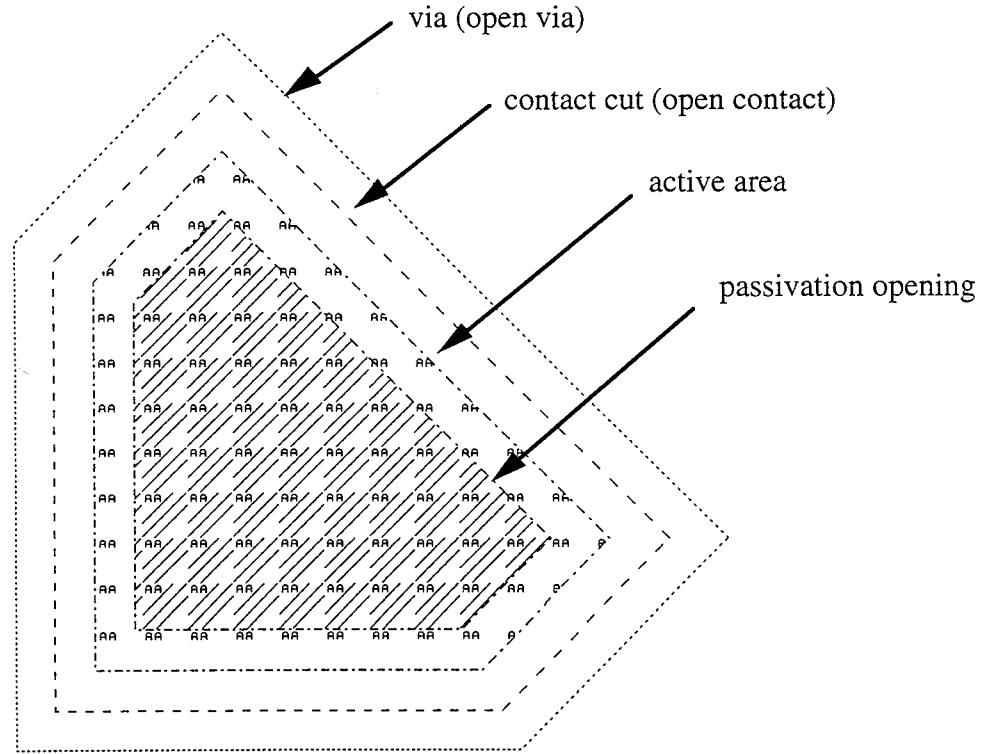
*Fig. 2.2.3.2.1.4. Superposition of the masks to define an exposed silicon area.*
