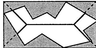
Fig. 2.2.3.2.1.2. Pyramid formed in the silicon etched through a mask of any form.
