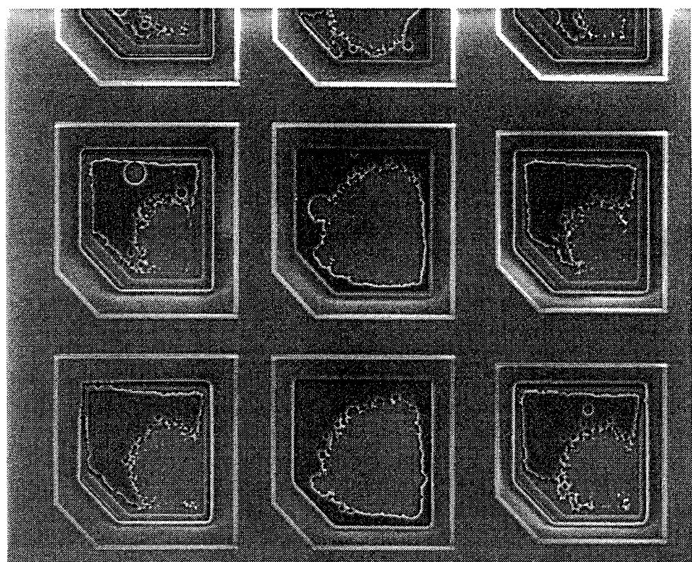
Fig. 2.2.3.3.2.2. Residual silicon dioxide remaining in the open areas after the CMOS processing
