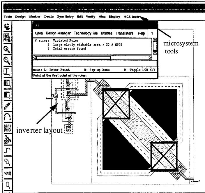
*Fig. 3.4.3.3. Prédiction of a post-process etching problem*
