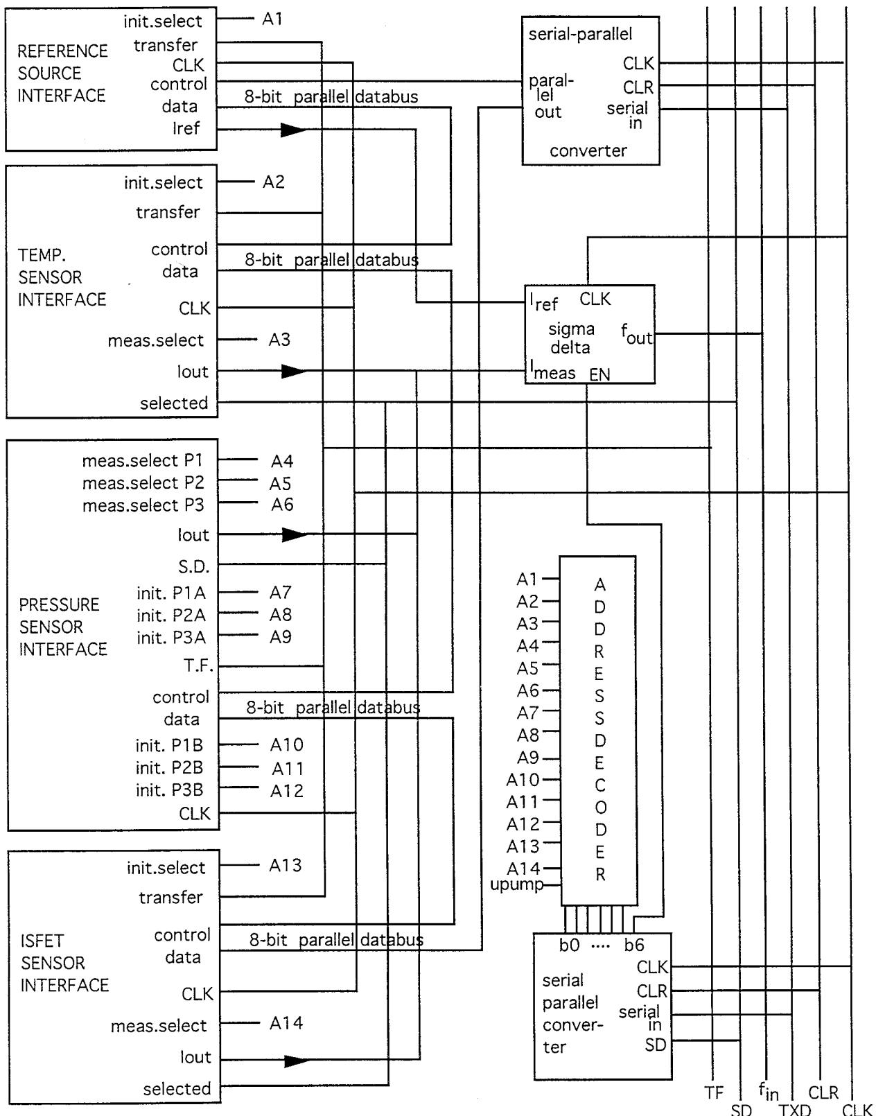
Fig. 4.3.4.1.1. System level configuration of the BARMINT sensor module
