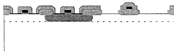
Step 12 : Metal 1 deposition and etching
