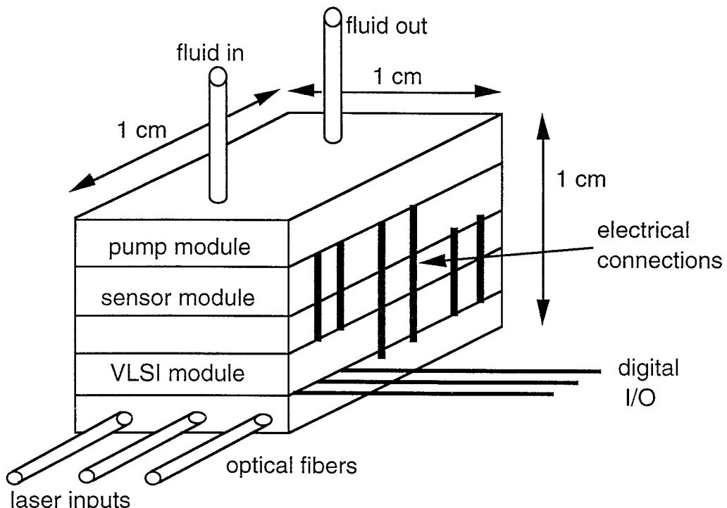
*Fig. 4.2.1.1.3. Physical dimensions of the BARMINT microsystem*
