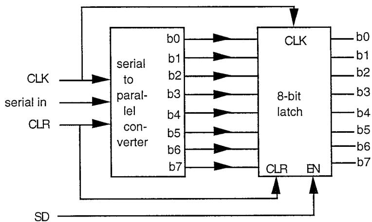
Fig. 4.3.4.4.3. Address serial-to-parallel converters for the BARMINT microsystem
