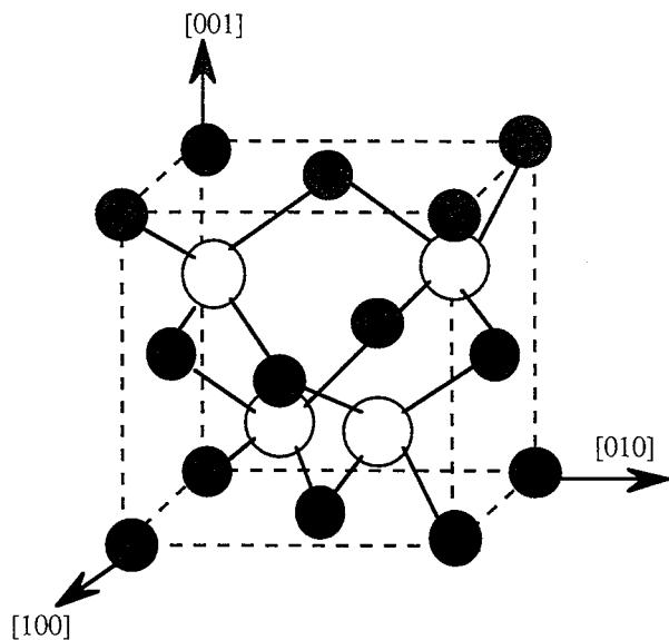
Fig. 2.3.1.1.1. Conventional unit cube for GaAs, zinc blende structure
