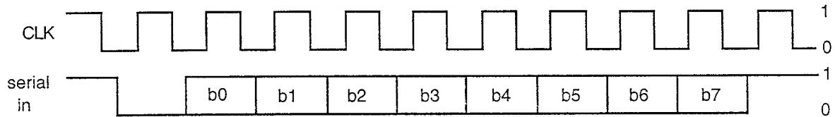
Fig.4.3.4.4.2. Input signals for the serial-to-parallel converter
