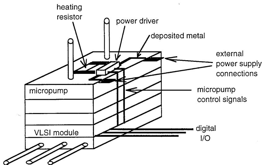
*Fig. 4.2.2.4.2. The power supply of the micropump in the BARMINT microsystem*
