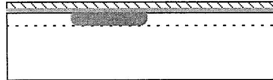
Step 7 : - Photoresist deposition, active zone exposure,
