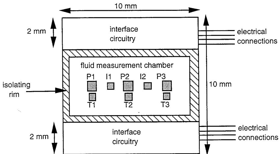
Fig. 4.2.1.3. Top view of the sensor module
