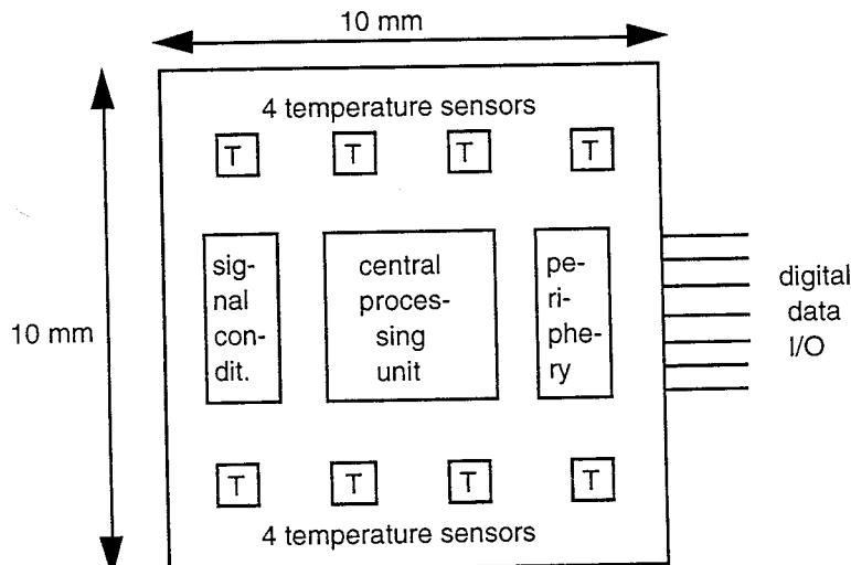
*Fig. 4.2.1.4.1. Top view of the VLSI module*
