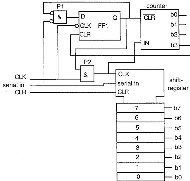
Fig.4.3.4.4.1. Schematic of the serial-to-parallel converter
