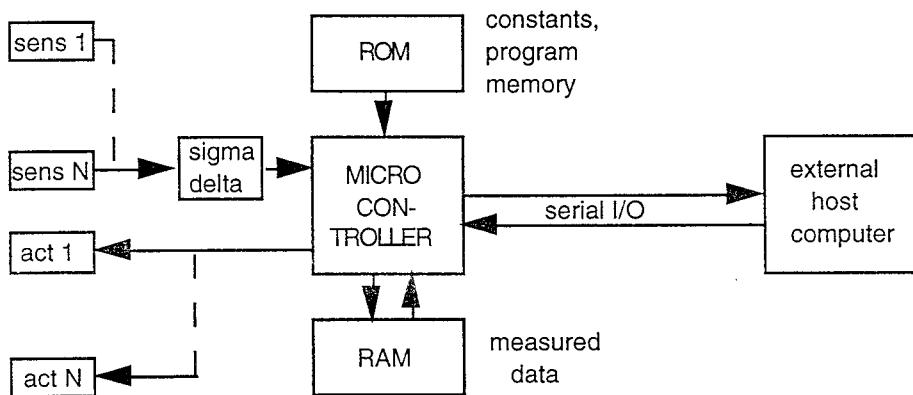
*Fig. 4.3.1.1.1. Position of the microcontroller within a microsystem*
