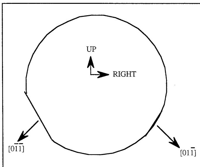
Fig. 2.3.2.3.1.1. The (100) GaAs wafer orientation compared with the layout window in CADENCE (up and right)
