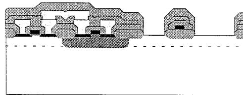
**Step 18 : Silicon etching (post-processing operation)**
