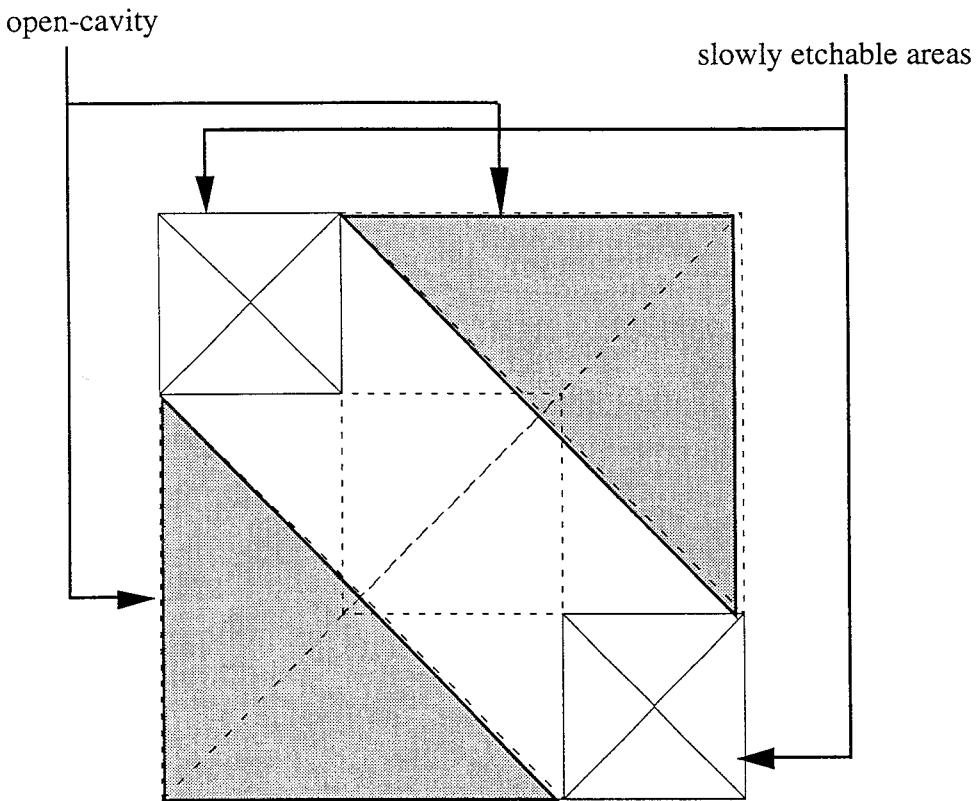
*Fig. 2.2.3.2.2.1. auto generation of the open-cavities (each open-cavity is attached to one open area) and of the slowly etchable areas (areas that may be difficult to etch in normal etching conditions)*
