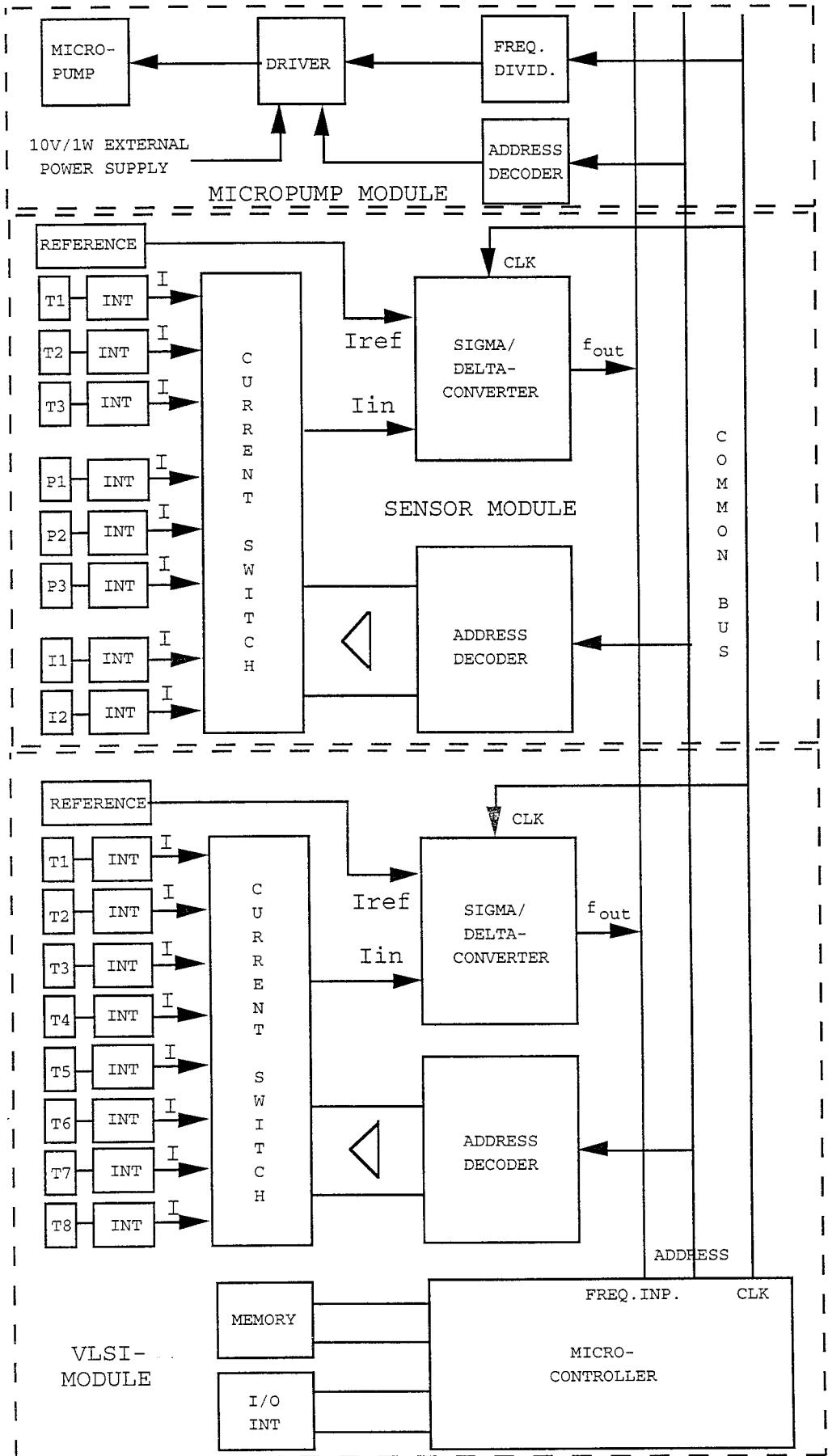
Fig. 4.2.2.5.1. The concept for the electrical configuration of the BARMINT microsystem
