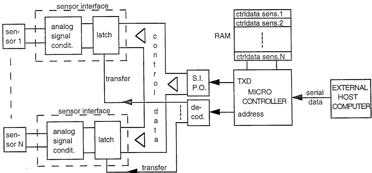
Fig. 4.3.3.1.1. The transfer of compensation control data from host to sensor interfaces
