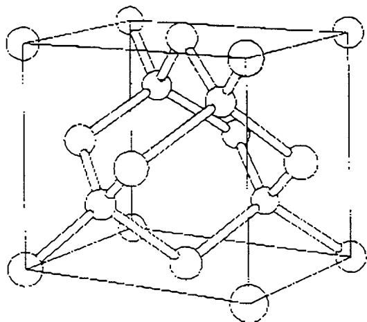
*Fig. 2.2.1.1. Silicon crystal lattice*
