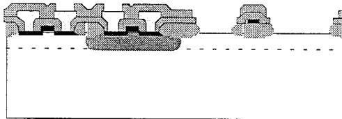
Step 15 : Metal 2 deposition and etching
