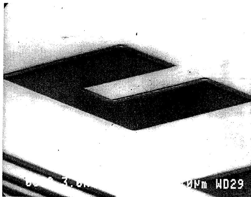
*Fig. 2.2.3.3.3.1.1. SEM photograph of a free-standing silicon dioxide cantilever structure containing piezo-resistive polysilicon lines*
