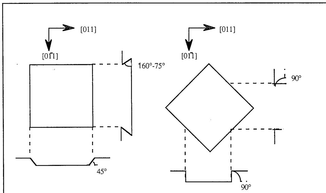
*Fig. 2.3.2.2.1.2. The appearance of etched wall for reaction-rate-limited etching on (100) GaAs*
