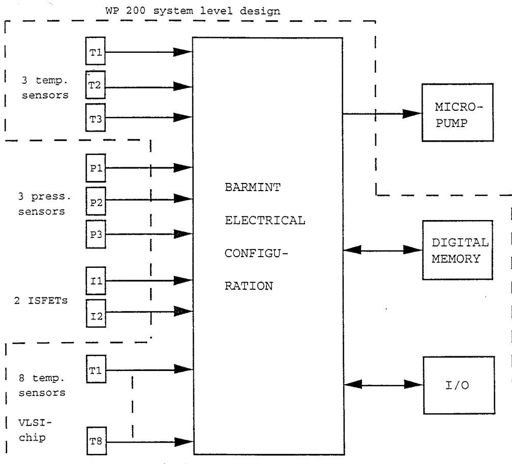
*Fig. 4.2.2.1. BARMINT electrical system level architecture*
