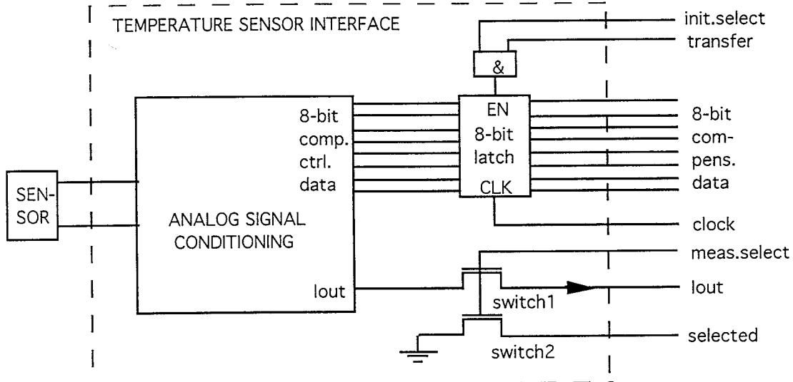
Fig. 4.3.3.3.1. Completely equipped BARMINT temperature sensor interface module
