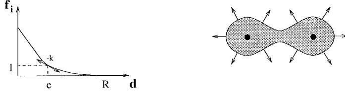
Figure 1: Field generated by two points, and the resulting implicit surface.
