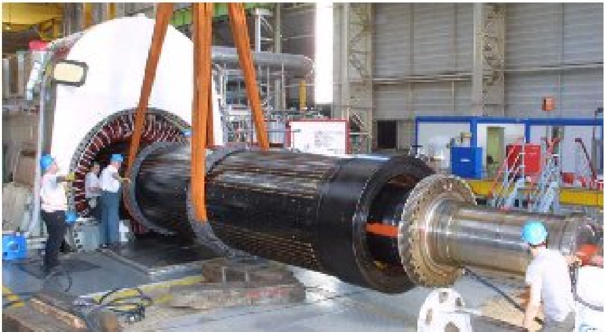
Figure 2: 2-poles rotor of turbogenerator
