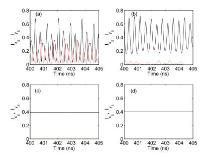
**Figure 8.3.11**: Time-traces of the x-LP (black) and y-LP (red) slave laser mode intensities for different values of the spin-flip relaxation rate parameter: (a)  $\gamma_s = 10 \text{ ns}^{-1}$ , (b)  $\gamma_s = 30 \text{ ns}^{-1}$ , (c)  $\gamma_s = 40 \text{ ns}^{-1}$ , (d)  $\gamma_s = 300 \text{ ns}^{-1}$ .
