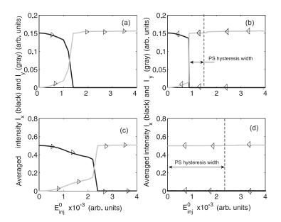
**Figure 4.4.2**: Hysteresis in the polarization resolved averaged intensity of the VCSEL for two values of the bias currents: 1)  $\mu = 1.15$  when increasing (a) and then decreasing (b) the injection strength  $E_{inj}^0$ ; 2)  $\mu = 1.5$  when increasing (c) and then decreasing (d) the injection strength  $E_{inj}^0$ . The frequency detuning is fixed at  $\Delta \omega = 3$  rad.ns<sup>-1</sup>. Black (gray) represents the low- (high-) frequency x-(y-) LP mode
