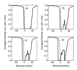
**Figure 4.5.9**: Effect of the linewidth enhancement factor  $\alpha$  on the polarization bistability induced by frequency detuning. The averaged x-LP mode intensity is plotted as a function of the detuning, for a fixed injection strength  $(P_{inj}/I_0 = 0.09\%)$  and for increasing values of  $\alpha$ : (a)  $\alpha = 3.4$ , (b)  $\alpha = 3.9$ , (c)  $\alpha = 4.3$ , (d)  $\alpha = 5.0$ .
