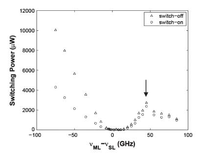
**Figure 4.2.4**: Evolution of the switching off (triangle) and switching on (circle) power when the injected power is increased and decreased respectively and this for different frequency detunings between master and slave lasers,  $\Delta \nu = \nu_{ML} - \nu_{SL}$ . The arrow indicates the onset of the locking of the VCSEL first order transverse mode to the master laser which is associated with a strong depression of the fundamental transverse mode
