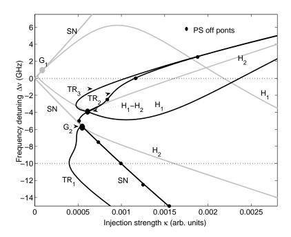
**Figure 6.3.1**: Bifurcation diagram of the two-mode model in the  $(\kappa, \Delta \nu)$  plane. Black (grey) denotes supercritical (subcritical) bifurcation. The dotted lines indicates the bifurcation scenarios analyzed in Fig. 6.3.2 and detailed in Fig. 6.3.3 and Fig. 6.3.4.
