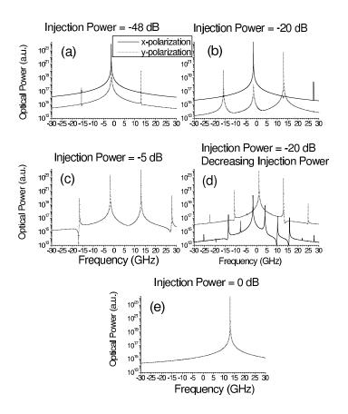
**Figure 7.2.4**: Polarization resolved optical spectra for several values of the injected power when the frequency detuning is 13 GHz. x- and y-polarized spectra are plotted with solid and dotted lines, respectively. (a), (b), (c), and (e) correspond to increasing injection power while (d) corresponds to decreasing power. Zero frequency corresponds to injection at the central frequency between the two polarizations of the fundamental mode.
