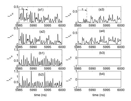
**Figure 8.2.1**: Time-traces of master and slave laser LP mode intensities for  $\eta = f = 6$  ns<sup>-1</sup>: (a1-a4) chaos in both x- and y-LP modes and (b1-b4) single-mode chaos.
