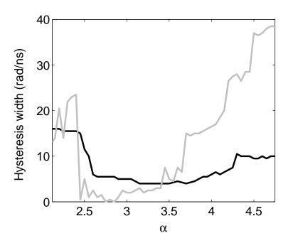
**Figure 4.5.8**: Influence of the linewidth enhancement factor  $\alpha$  on the width of the hysteresis associated with the LF-PS point, for either a weak (black)  $(P_{inj}/I_0 = 0.09\%)$  or large (gray)  $(P_{inj}/I_0 = 1.50\%)$  injection strength.
