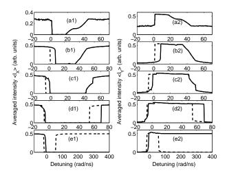
**Figure 4.5.10**: Effect of the spin-flip relaxation rate  $\gamma_s$  on the polarization bistability induced by frequency detuning. The averaged x LP mode (left) and y LP mode (right) intensities are plotted as a function of the detuning, for a fixed injection strength  $(P_{inj}/I_0 = 0.09\%)$  and for increasing values of  $\gamma_s = (a1), (a2)$  1; (b1), (b2) 20; (c1), (c2) 50; (d1), (d2) 75; and (e1), (e2) 100  $ns^{-1}$ .
