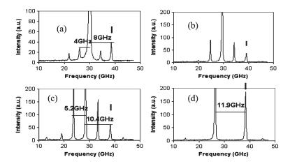
**Figure 5.3.1**: Polarization-resolved optical spectra of the VCSEL subject to optical injection at a frequency detuning of 10 GHz and increasing the injected power  $P_{inj}$ : (a)  $P_{inj} = 29\mu W$ . (b)  $70\mu W$ . (c)  $251\mu W$ . (d)  $800\mu W$ . (a)-(c) Subharmonic resonances with wave mixing. (d) Represents a limit cycle dynamics (period-one). Only vertical polarization is represented. The vertical line denotes the ML frequency.
