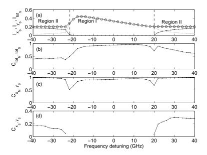
**Figure 8.3.1**: Evolution of the time-averaged LP mode and total intensities in the slave laser (a), of the correlation coefficient  $C_{tot_M,tot_S}$  (b),  $C_{x_M,y_S}$  (c),  $C_{x_S,y_S}$  (c) as function of the frequency detuning, for a fixed injection rate  $\eta = 100$  GHz. Parameters are specified in the text.
