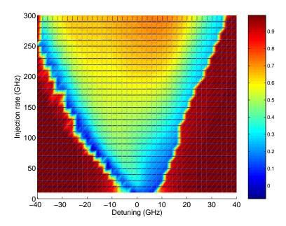
**Figure 8.3.6**: Mapping of correlation coefficient  $C_{x_M,y_S}$  at zero time-lag between the time-traces corresponding to master x-LP mode and to slave y-LP mode, in the plane of the injection parameters.
