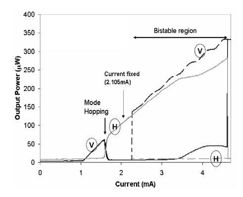
Figure 4.2.2: Polarization-resolved optical power versus injection current curve of the solitary VCSEL for a substrate temperature of  $20^{\circ}$  C. The lines corresponding to the vertical and horizontal polarization are indicated by V and H, respectively. The continuous (dashed) line represents the upward (downward) scan.
