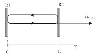
Figure 2.1.3: Schematic view of a Fabry-Perot resonator.
