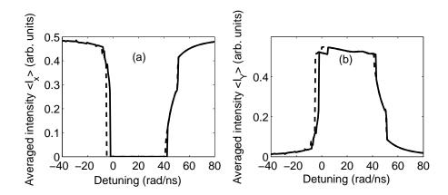
**Figure 4.5.2**: Pure frequency polarization bistability induced by optical injection. Solid (dashed) line represents the evolution of the averaged optical intensity when the frequency detuning is increased from negative to positive values (decreased from positive to negative values) and for a fixed injection strength  $P_{inj}/I_0 = 0.09\%$ : (a) x-polarized mode, (b) y-polarization direction.
