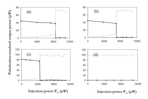
**Figure 4.2.3**: Hysteresis in the polarization resolved optical power of the VCSEL when the injected power  $P_{inj}$  is first increased and then decreased for two values of the bias current  $I_{SL}$ . The black (gray) line represents the horizontal (vertical) polarization.  $I_{SL} = 1.9$  mA and for  $\Delta \nu = -36$  GHz: (a) Increasing  $P_{inj}$ , (b) Decreasing  $P_{inj}$ ;  $I_{SL} = 2.603$  mA and for  $\Delta \nu = -20$  GHz: (c) Increasing  $P_{inj}$ , (d) decreasing  $P_{inj}$ .
