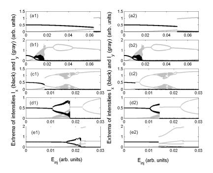
**Figure 6.2.1**: Bifurcation diagrams of the LP mode intensities showing the different scenarios of PS for (a)  $\Delta \omega = 72$ ; (b) 30; (c) 23; (d) 10; and (e)  $-2.2 \text{ rad.ns}^{-1}$ . Left panels: injection strength is increased; right panels: injection strength is decreased. Black (grey) corresponds to x- (y-) LP mode. The linewidth enhancement factor is  $\alpha = 3$ .
