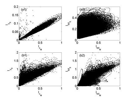
**Figure 8.3.4**: Synchronization diagrams corresponding to regions II [(a1), (a2)] and I [(b1), (b2)] of qualitatively different synchronization properties: (a1), (b1)  $I_{y_S}$  as function of  $I_{x_M}$ , (a2), (b2)  $I_{tot_S}$  as function of  $I_{tot_M}$ .
