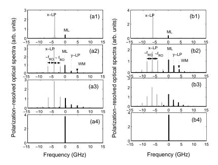
**Figure 6.2.8**: Theoretical polarization-resolved optical spectra showing the dynamics leading to PS and locking when increasing the injection strength (from top to bottom) for: (a1)-(a4)  $\Delta \omega = -2.2 \text{ rad.ns}^{-1}$  and (b1)-(b4)  $\Delta \omega = 10 \text{ rad.ns}^{-1}$ . Black (grey) corresponds to y- (x-) LP mode.
