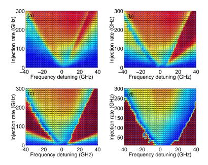
**Figure 8.3.9**: Mapping of correlation coefficient  $C_{x_M,y_S}$  at zero time-lag between the time-traces corresponding to master x-LP mode and to slave y-LP mode, in the plane of the injection parameters with different values of the spin-flip relaxation rate parameter: (a)  $\gamma_s = 10 \text{ ns}^{-1}$ , (b)  $\gamma_s = 30 \text{ ns}^{-1}$ , (c)  $\gamma_s = 40 \text{ ns}^{-1}$ , (d)  $\gamma_s = 300 \text{ ns}^{-1}$ .
