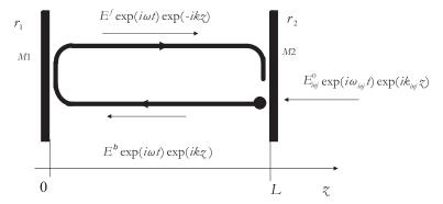
**Figure A.0.1**: Schematic of a Fabry-Perot cavity for the modelling of a semiconductor laser under optical injection. The superscripts f and b denote the forward and backward internal travelling field wave.
