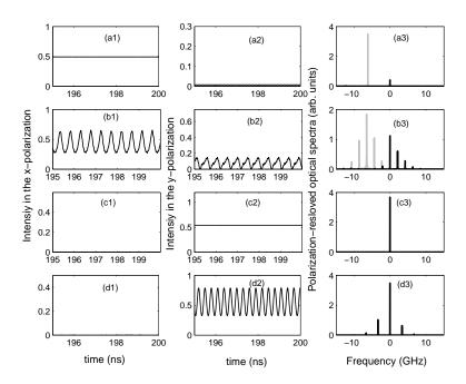
Figure 6.2.5: Polarization-resolved intensities and optical spectra at  $\Delta \omega = 10 \text{ rad.ns}^{-1}$  corresponding to Fig. 6.2.1(d) showing for: (a)  $E_{inj} = 0.005$ , weak injection regime, (b)  $E_{inj} = 0.013$ , excitation of limit cycle before PS for the x-LP mode and wave mixing between y-LP and ML; (b)  $E_{inj} = 0.020$ , injection locking; (c)  $E_{inj} = 0.025$ , limit cycle after crossing a Hopf bifurcation. In the spectra, black (grey) corresponds to y- (x-) LP mode.
