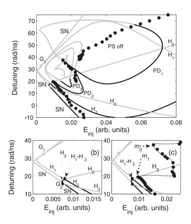
**Figure 6.2.9**: Bifurcation diagram in the plane  $(E_{inj}, \Delta \omega)$  for  $\alpha = 3.75$ . Black (grey) denotes supercritical (subcritical) part of each bifurcation curve. Bifurcation curves, codimension-two points, and switching points keep the same meaning as in Fig. 6.2.7.
