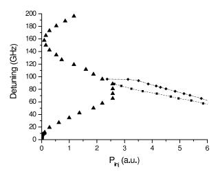
**Figure 7.4.1:** Injection power required for PS in a VCSEL subject to orthogonal optical injection. Switching from x- to y-polarization when increasing the injection power is shown with triangles. The injection power required for the  $LP_{11,y}$  modal power to reach an appreciable value, 0.5, has been plotted if  $P_{inj}$  is increased (diamonds) and if  $P_{inj}$  is decreased (squares). Parameters correspond to those in Fig.7.2.2(a).
