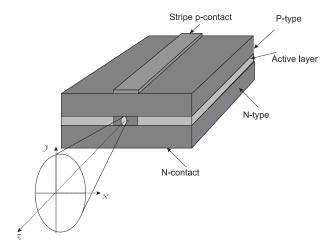
Figure 2.1.1: Schematic view of an edge-emitting laser.
