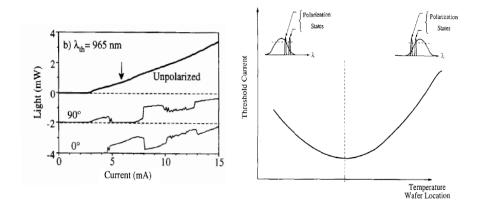
**Figure 3.1.1**: Polarization switching in VCSEL as an effect of current heating (left). Illustration of the redshift in both the material and polarization-resolved modal gain (right).  $0^{\circ}$  and  $90^{\circ}$  denotes the two orthogonal polarization states, after [36].
