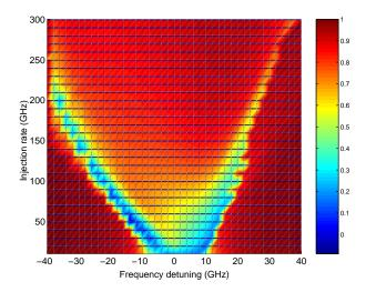
**Figure 8.3.8**: Mapping of correlation coefficient  $C_{x_M,y_S}$  at zero time-lag between the time-traces corresponding to master x-LP mode and to slave y-LP mode, in the plane of the injection parameters with no mismatch between the values of linear cavity anisotropies in slave and master VCSELs.
