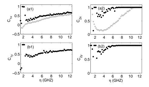
**Figure 8.2.2**: Evolution of the correlation coefficients related to isochronous (a1 and b1) and anticipative (a2 and b2) synchronization as a function of  $\eta$ . The gray (black) color corresponds to the case of single-mode (two-mode) chaos.
