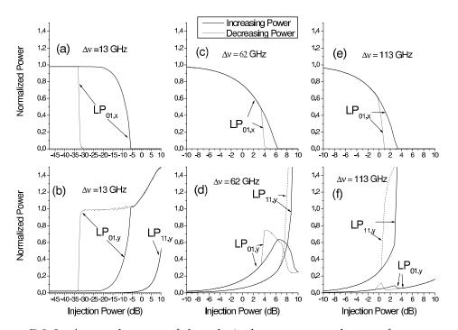
**Figure 7.2.3**: Averaged powers of the polarized transverse modes as a function of the injection power. The upper (lower) part of the figure corresponds to x- (y-) polarized light. First, second, and third columns correspond to 13, 62, and 113 GHz frequency detunings, respectively. Results obtained when increasing (decreasing) the injection power are plotted with solid (dotted) lines.
