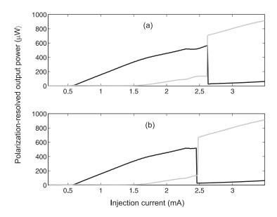
**Figure 3.3.1**: Experimental polarization-resolved averaged Light-Current characteristic of  $VCSEL_1$  when the injection current is first increased (a) and then decreased (b). Black (gray) represents the averaged power for low-(high) frequency mode. The temperature has been stabilized at  $20^{\circ}$  C.
