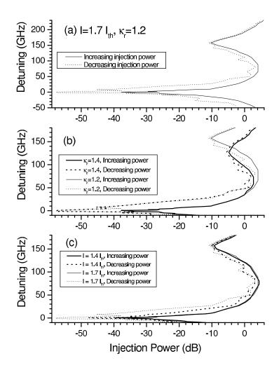
**Figure 7.2.2**: Injection power required for PS in a VCSEL subject to orthogonal optical injection. Switching from x to y (y to x) polarization when increasing (decreasing) the injection power is shown with solid (dotted) lines. (a) Corresponds to  $I=1.7I_{th}$  and  $\kappa_r=1.2$ . (b) Results for  $I=1.7I_{th}$  and  $\kappa_r=1.4$ . (c) Rresults for  $I=1.4I_{th}$  and  $\kappa_r=1.2$ .
