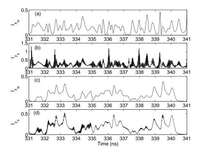
**Figure 8.3.10**: Time traces of the x-LP master laser intensity and y-LP slave laser intensity for  $\eta = 200$  GHz,  $\Delta \omega / 2\pi = 30$  GHz and for two different values of the spin-flip relaxation rate parameter: (a), (b)  $\gamma_s = 10 \text{ ns}^{-1}$  and (c), (d)  $\gamma_s = 40 \text{ ns}^{-1}$ .
