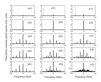
**Figure 6.2.11**: Theoretical polarization-resolved optical spectra showing the dynamics leading to PS and locking when increasing the injection strength (from top to bottom) for: (a1)-(a5)  $\alpha = 2.25$  and  $\Delta\omega = 26.6$  rad.ns<sup>-1</sup>; (b1)-(b5)  $\alpha = 3$  and  $\Delta\omega = 23$  rad.ns<sup>-1</sup>; (c1)-(c5)  $\alpha = 3.75$  and  $\Delta\omega = 17.3$  rad.ns<sup>-1</sup>. Black (grey) corresponds to y- (x-) LP mode.
