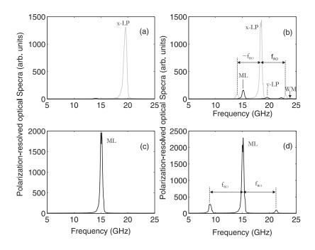
**Figure 5.4.4**: Polarization-resolved optical spectra showing dynamics of the VCSEL subject to optical injection at a frequency detuning of -4.1 GHz and increasing the injected power  $P_{inj}$ : (a)  $P_{inj} = 19 \mu W$ ; (b) 88  $\mu W$ ; (c) 114  $\mu W$ ; (d) 236  $\mu W$ . Black (gray) represents vertical (horizontal) mode.
