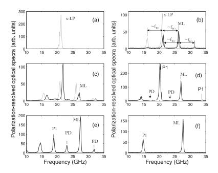
**Figure 5.4.3**: Polarization-resolved optical spectra showing dynamics of the VCSEL subject to optical injection at a frequency detuning of 4.4 GHz and increasing the injected power  $P_{inj}$ : (a)  $P_{inj} = 3 \mu W$ ; (b)  $83 \mu W$ ; (c)  $185 \mu W$ ; (d)  $265 \mu W$ ; (e)  $558 \mu W$ ; (f)  $3454 \mu W$ .  $P_1$  denotes a period-one limit cycle while PD denotes period doubling features. Black (gray) represents vertical (horizontal) mode.
