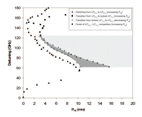
**Figure 7.3.1**: Experimental mapping of PS and transverse modes competition in the plane detuning versus injection power  $(P_{inj})$ . The bias current and the operating temperature are fixed at 2.105 mA and 20° C, respectively.
