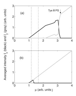
**Figure 4.4.1**: Theoretical polarization-resolved Light-Current characteristics of the free-running VCSEL when the normalized injection current  $\mu$  is first increased (a) and then decreased (b). Black (gray) represents the low-(high-) frequency x-(y-) LP mode.
