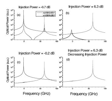
**Figure 7.2.5**: Polarization resolved optical spectra for several values of the injected power when the frequency detuning is 62 GHz. x and y-polarized spectra are plotted with solid and dotted lines, respectively. (a)-(c) correspond to increasing injection power while (d) corresponds to decreasing power.
