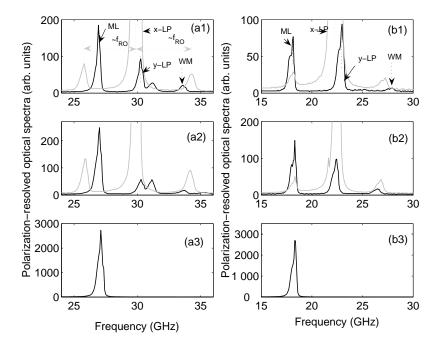
**Figure 5.4.1:** Experimental polarization-resolved optical spectra of VCSEL<sub>2</sub> showing the dynamics leading to PS and locking when increasing the injection power for two detuning values: (a1)-(a3) for  $\Delta \nu = -3.45$  GHz and (b1)-(b3) for  $\Delta \nu = -5.37$  GHz. Black (grey) corresponds to vertical y- (horizontal x-) LP mode.
