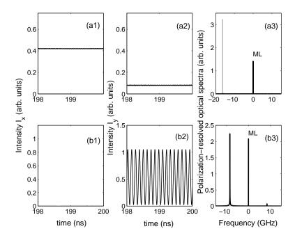
**Figure 6.2.2**: Polarization-resolved intensities and optical spectra corresponding to the case of abrupt PS at  $\Delta \omega = 70 \text{ rad.ns}^{-1}$  in Fig. 6.2.1(a). (a)  $E_{inj} = 0.04$ , before PS; (b)  $E_{inj} = 0.07$ , after PS. In the spectra black (grey) corresponds to y- (x-) LP mode.
