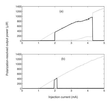
**Figure 3.3.2**: Experimental polarization-resolved averaged Light-Current characteristic of  $VCSEL_2$  when the injection current is first increased (a) and then decreased (b). Black (gray) represents the averaged power for low-(high) frequency mode. The temperature has been stabilized at  $20^{\circ}$  C.
