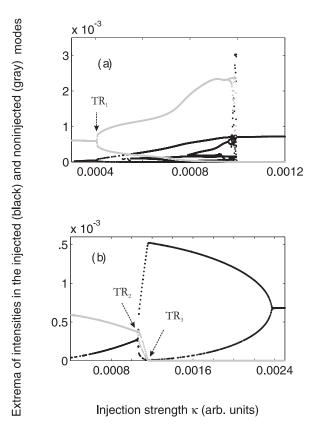
**Figure 6.3.2**: Bifurcation diagram showing the maxima and minima of the intensities of the injected mode (black) and the noninjected mode (gray) as a function of the injection strength,  $\kappa$ , when the detuning is fixed at: (a)  $\Delta \nu = -10$  GHz and, (b)  $\Delta \nu = 0$  GHz.
