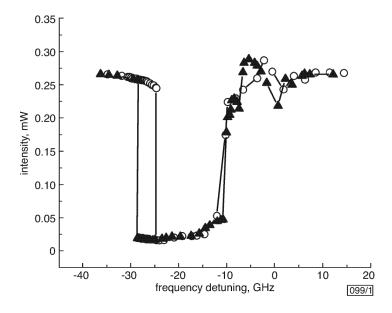
**Figure 4.5.1**: Intensity of X-component of slave laser light polarization as function of frequency detuning, after [132]
