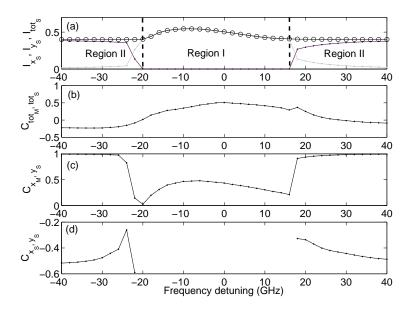
**Figure 8.3.5**: Same as Fig. 8.3.1 but considering mismatch in VCSEL linear cavity anisotropies and injection currents:  $\gamma_{a_M} = 0.1$ ,  $\gamma_{p_M} = 6$  rad/ns,  $\mu_M = 1.2$  and  $\gamma_{a_M} = -0.1$ ,  $\gamma_{p_M} = 8.5$  rad/ns,  $\mu_M = 1.4$
