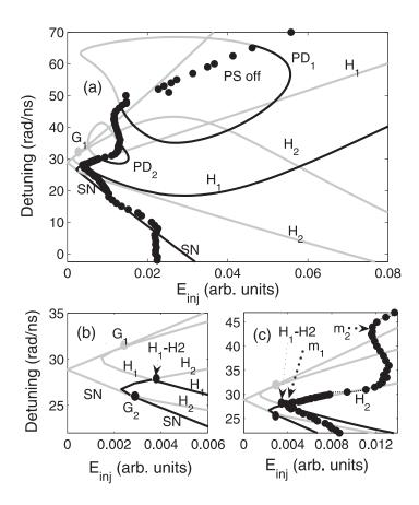
Figure 6.2.10: Bifurcation diagram in the plane  $(E_{inj}, \Delta\omega)$  for  $\alpha = 2.25$ . Black (grey) denotes the supercritical (subcritical) part of each bifurcation line. Bifurcation curves, codimension-two points, and switching points keep the same meaning as in Fig. 6.2.7.
