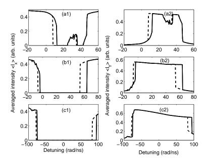
**Figure 4.5.3**: Influence of the injection strength on pure-frequency polarization bistability. Same as Fig. 1 but for (a1), (a2):  $P_{inj}/I_0 = 0.05\%$ , (b1), (b2):  $P_{inj}/I_0 = 0.15\%$ , (c1), (c2):  $P_{inj}/I_0 = 1.5\%$ .
