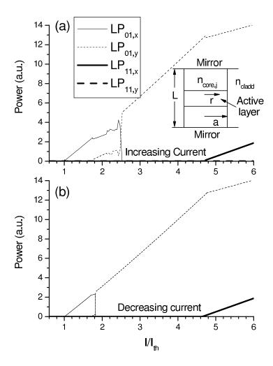
Figure 7.2.1: (a) Light-current characteristics of a multimode VCSEL without optical injection. This figure is obtained by fixing  $k_{ij} = 0$ ,  $\kappa_r = 1.2$ , and by increasing linearly the value of the current I from  $0.1I_{th}$  to  $6I_{th}$  during  $10\mu s$ . (b) L-I characteristics when decreasing the current from  $6I_{th}$  to  $0.1I_{th}$ during  $10\mu s$ . The inset of Fig. 7.2.1(a) shows an schematic diagram of the VCSEL.
