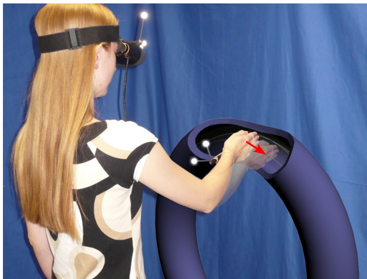
Figure 1-3: Compositing of a user reaching into a virtual force field, including the visualised hand displacement to the right.
