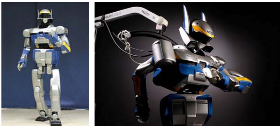
Figure 4.8: HRP-2, a humanoid robot. HRP-2 is 154 cm tall, and weights 58 kg with batteries. It has over 30 DOFs and is equipped for both stereo vision and force sensing.
