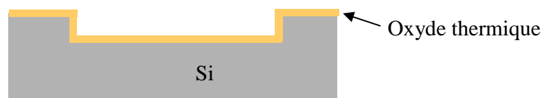
Figure 3-1 : process flow Nanomag : caisson Si (Nanomag process flow: patterning of Si substrate)
