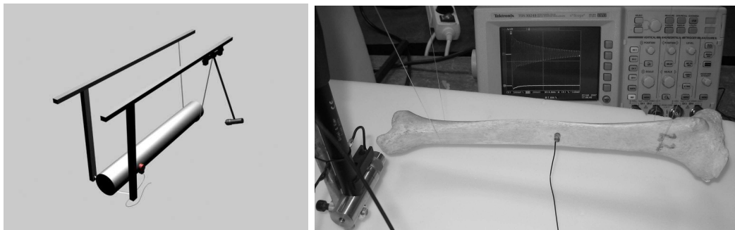
FIG. 22.3 – (a) The impact experiment. The hammer strikes the cylinder sideways and the response is measured using the accelerometer. (b) Photograph of the human tibia, hammer impact and vibration experiment. The bone is suspended on a test rig using nylon threads and the impact is applied sideways on the medial malleolus to generate flexural waves. The response is measured at the center of the bone using a featherweight (0.75 gram) accelerometer (Brüel and Kjaer B&K4374).
