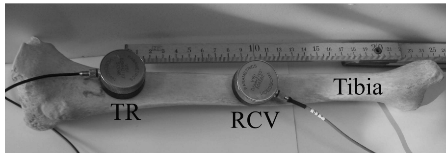
FIG. 22.9 – Photograph of the shear wave velocity measurement experiment. The transmitter (TR) remains at a fixed position while the receiver (RCV) is displaced in 2.0 cm steps.
