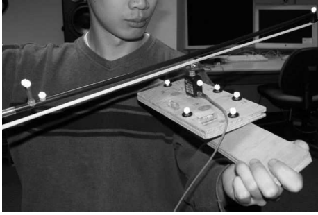
FIG. 12. Load cell mounted on wooden board used for bow force calibration. Bow position is obtained by motion capture.
