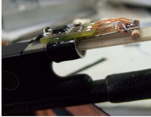
Fig. 7: Bow force sensor. A thin steel strip is clamped to the flat side of the ferrule. The strip bends as the deflected bow hair presses at the free end via a wooden bearing piece. The bending is measured by two strain gauges glued to the strip. A Wheatstone bridge and conditioning amplifier is integrated in the sensor.
