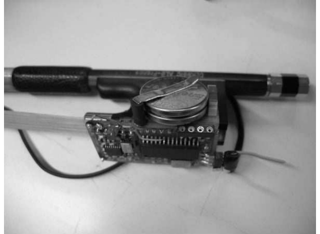
FIG. 1. Module placed at the frog of the violin bow to measure players' bowing movements. It consists of two accelerometers and a RF transmitter, powered with batteries.
