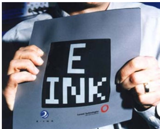
Figure 2.21: Electronic paperlike display showing two different images. The device consists of several hundred pixels controlled by a flexible active matrix backplane circuit formed by microcontact printing. The relatively coarse resolution of the display is not limited by material properties or by the printing techniques. Instead, it is set by practical considerations for achieving high pixel yields in the relatively uncontrolled environment of the chemistry laboratory in which the circuits were fabricated.
