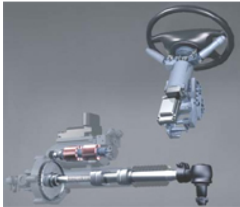
Figure 2.3: Steer by wire system.
