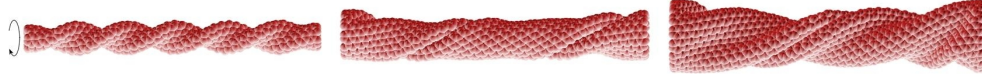
Figure 3.12 – (Color online) Shape of three twisted chiral CNTs with the same length L = 9.6\text{nm} and the same chiral angle = 19.1^\circ , just before the fracture occurs, at \theta = 630^\circ , 497^\circ and 427^\circ , respectively. Left : (6, 3) , R = 0.31\text{nm} ; middle : (14, 7) , R = 0.72\text{nm} ; right : (20, 10) , R = 1.03\text{nm} .
