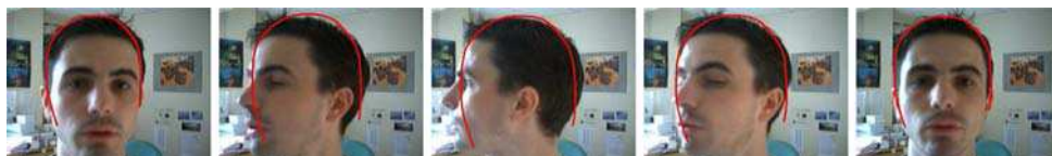
Fig. 17 Tracking scenario with CONDENSATION over a cluttered background. The red template depicts the MMSE estimate
