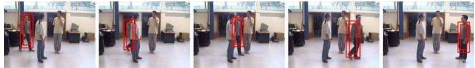
Fig. 36 A scenario involving persistent occlusions due to persons. Tracker based on a DMIF into the RBSSHSSIR algorithm
