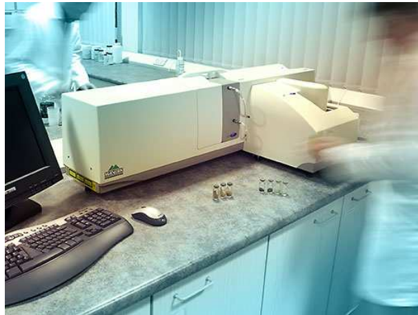
Figure I-21 : Malvern® MasterSizer 2000 (crédit photo Malvern Instruments, http://www.malverninstruments.fr )
