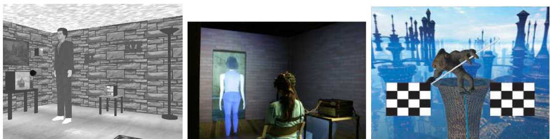
Figure 1.19: From left to right: manipulating electronic devices in a virtual flat with a P300-based BCI (picture from [Bay03]), controlling a virtual avatar by motor imagery (picture from [FLD + 07]), controlling the balance of a virtual monster using SSVEP (picture from [LKF + 05a]).
