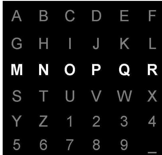
Figure 1.13: The P300 speller interface, as displayed on the user's screen [FD88].
