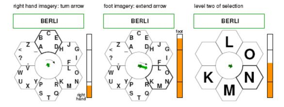
Figure 1.14: The interface of the "Hex-o-spell" application, as displayed on the BCI user's screen (picture from [BKD<sup>+</sup>07b]).
