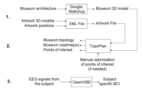
Figure 7.6: Software architecture for offline operations.
