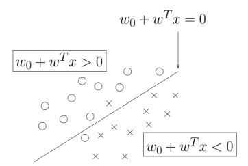
Figure 1.10: A hyperplane which separates two classes: the "circles" and the "crosses".
