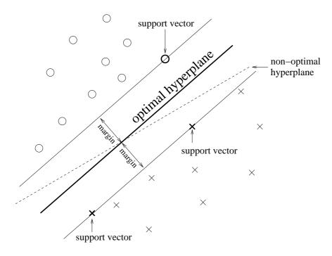
Figure 1.11: SVM find the optimal hyperplane for generalization.
