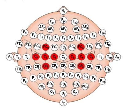
Figure 5.3: Placement of electrodes in the 10-10 international system. The electrodes we used in the experiment are displayed in red.
