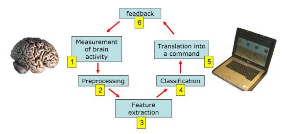
Figure 1: General architecture of an online brain-computer interface.
