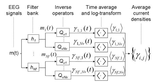
Figure 2.1: Computation of the average current densities  $\langle \gamma_{i,j} \rangle$  in all frequencies  $f_i$  and voxels  $v_j$ , from a training EEG record m(t).
