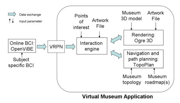
Figure 7.7: Software architecture for online operations.
