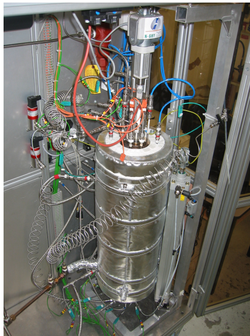
FIG. 3.4 – Heat exchanger - reformer unit designed by N-GHY .[Demand N-GHY if some explanations can be added to the picture.]
