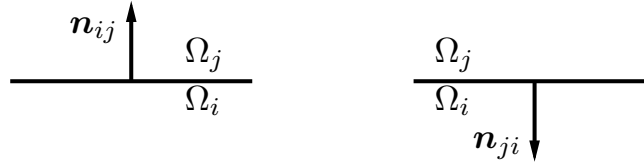
Figure 3.6: Normals for the definition of the traction unknowns.
