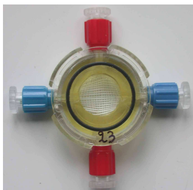
Figure 2 Hollow Fiber Bioartificial Liver bioreactor equipped with : semi-permeable (red connections) and oxygenation membranes (blue connections)
