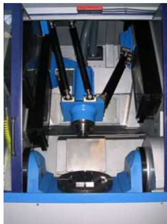
Figure 4.5 - Machine-outil Verne (Fondation Fatronik)
