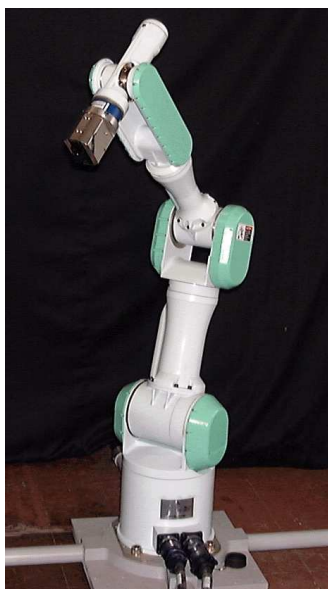
Figure 1.12 - Robot industriel sept axes PA 10 (Mitsubishi, Japon)
