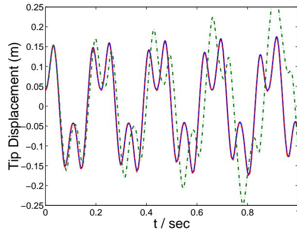
Figure 3.10: Time history of the transverse displacement at the tip of the beam for the system shown in figure 3.6, for initial conditions deduced from the initial values of the master coordinates  $a_1(0) = 0.63$ ,  $\phi_1(0) = 0.0$ ,  $a_2(0) = 0.38$ ,  $\phi_2(0) = 0.0$ . (—) time simulation of the reference model; (- - -) simulation of the reduced-order model; (- · - · -) results from the asymptotic expansion method.
