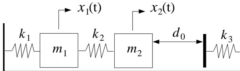
Figure 2.1: A two-degree of freedom piecewise linear system.
