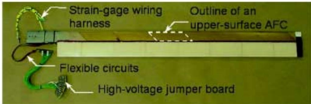
Figure 5.2: The prototype of the active twist rotor (ATR) blade [66]. AFC denotes the active fiber composites.
