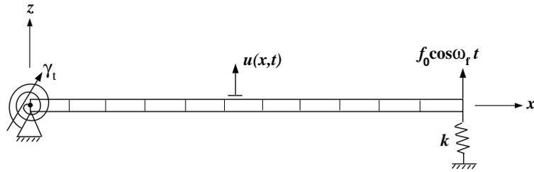
Figure 4.7: An Euler-Bernoulli beam with a nonlinear torsional spring,  $\gamma_t$ , at one end.
