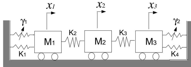
Figure 3.1: Schematic diagram of the mass–spring system: masses  $M_1 = M_2 = M_3 = 1$  kg; spring stiffnesses  $K_1 = 0.5$  N/m,  $K_2 = 5$  N/m,  $K_3 = 2.03$  N/m,  $K_4 = 0.6$  N/m; nonlinear spring forces  $\gamma_1 = 1.0 \times X_1(t)^3$  N,  $\gamma_2 = 1.5 \times X_3(t)^3$  N.  $X_1$ ,  $X_2$ , and  $X_3$  denote the displacements of masses  $M_1$ ,  $M_2$ , and  $M_3$  respectively.
