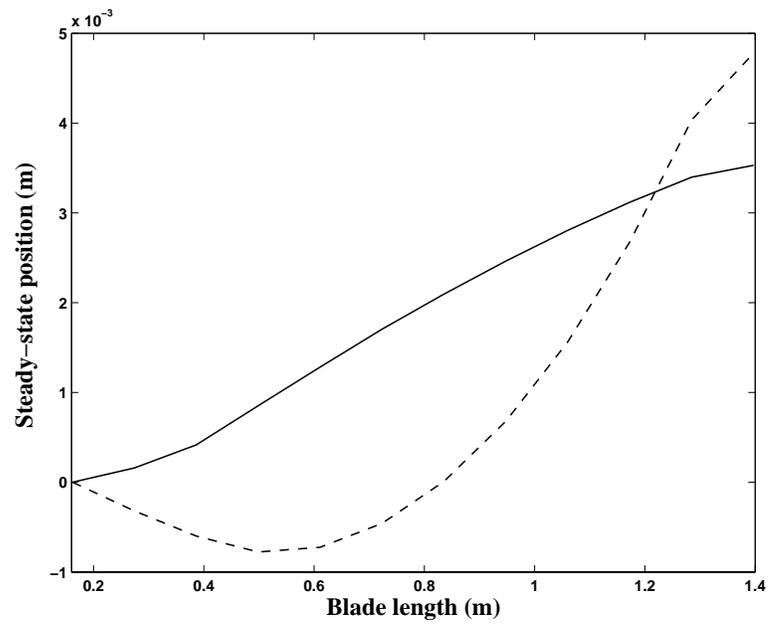
Figure 5.3: The steady-state equilibrium position of the ATR blade model. '—', the axial elongation  $u_{A1}$ ; '- - -', the lead-lag displacement  $u_{A2}$ .
