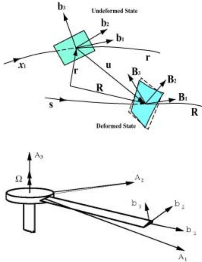
Figure 5.1: Schematic of the undeformed and deformed beam reference lines and cross-sections [64–66].
