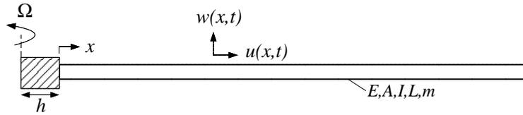
Figure 3.6: Schematic diagram of the rotating beam system. Rotating speed  $\Omega$  is constant. The uniform beam has the following material and geometrical parameters: Young's modulus  $E$ , cross sectional area  $A$ , second moment of cross sectional area  $I$ , length  $L$ , and mass per unit length  $m$ . The hub radius is  $h$ . (Abridged from reference [56].)
